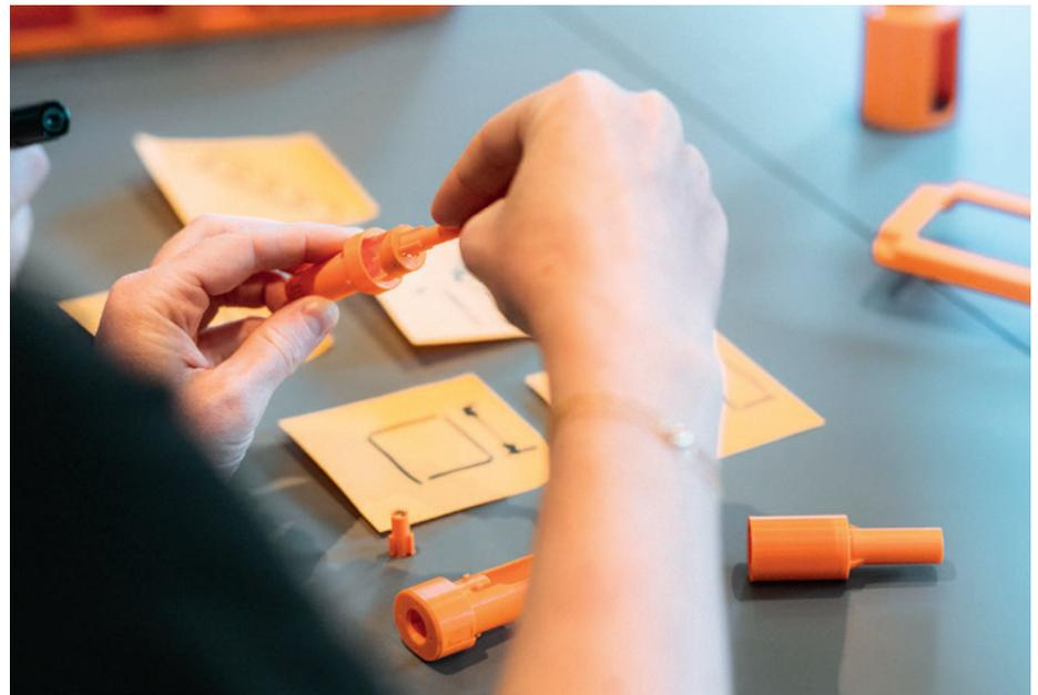
Figure 5: Hands-on evaluation of a device prototype with modular components – designing for easy disassembly supports more efficient recycling and sustainable end-of-life processing.
