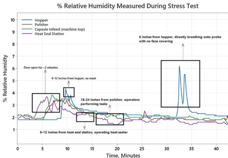
Figure 2: Relative humidity changes due to operator presence at various points in an ultra-low RH encapsulation suite.
