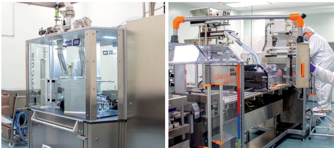
Figure 1: Commercial-scale encapsulation (Harro Höfliger Modu-C MS, left) and blistering (Pharmaworks TF2, right) within Catalent Boston.
