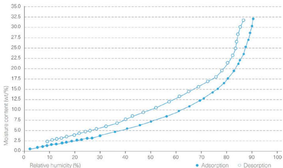
Figure 3: A DVS isotherm of an HPMC capsule.
