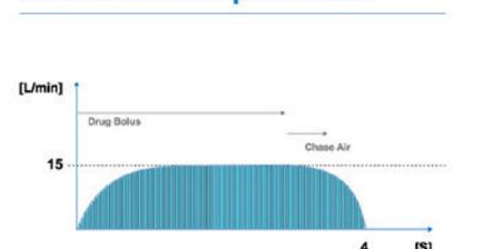
Figure 5: Kolibri's unique drug deposition optimisation through inspiratory flow control.
