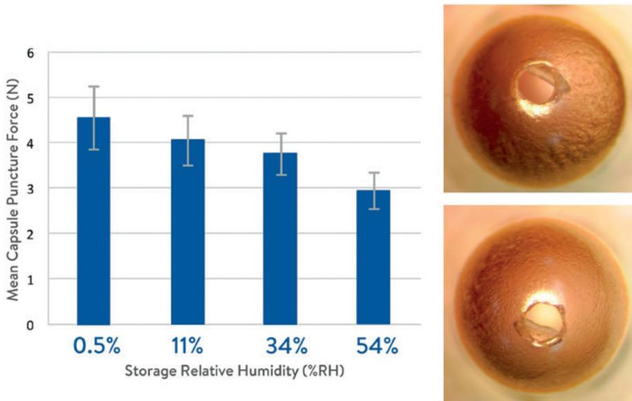
Figure 4: Puncture force change with various HPMC capsule storage conditions (left) and images of capsule punctures after 0.5% RH storage (right).
