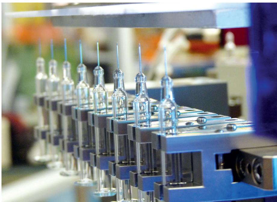
Figure 6: Glass syringe assembly line.
