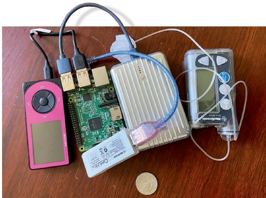
Figure 4: A DIY artificial pancreas system from 2016, using a battery-powered Raspberry Pi, Dexcom receiver, and CareLink USB stick transmitting to a Medtronic pump.<sup>16</sup>
