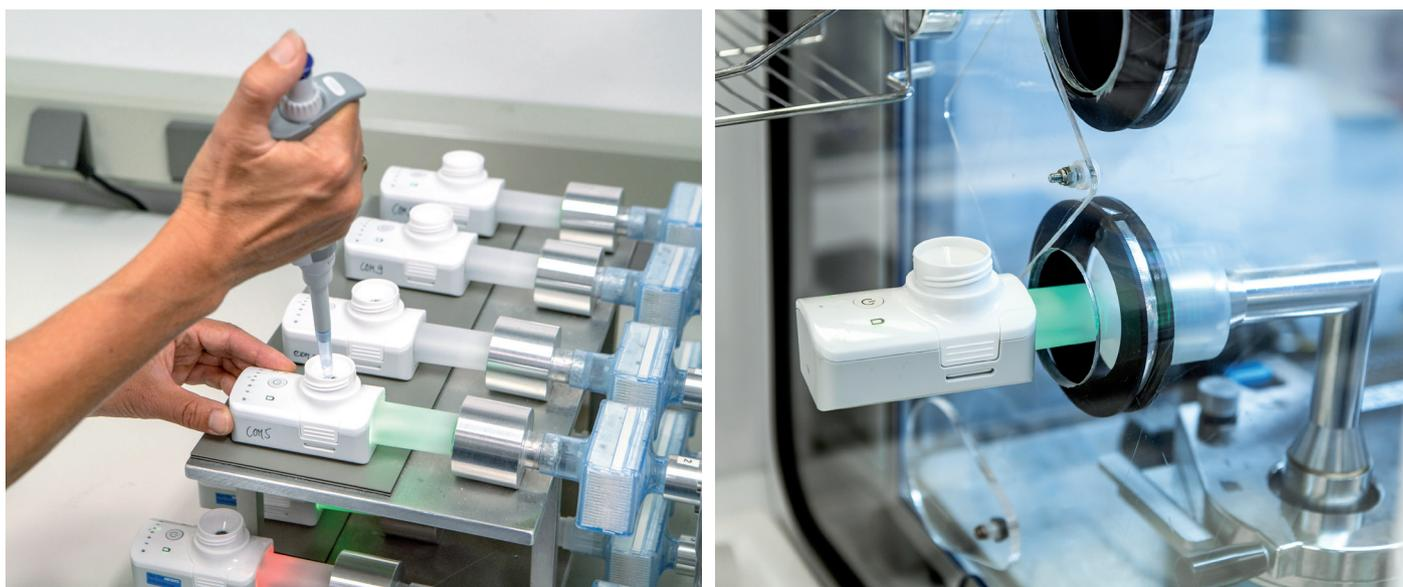
Figure 3: Vectura conducts extensive inhaler testing and analysis.
