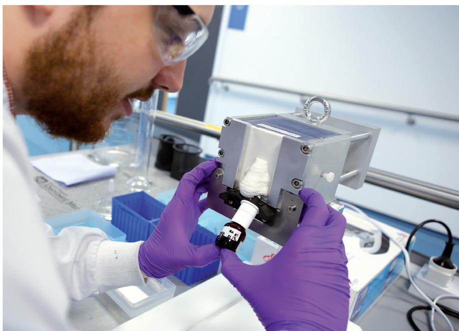
Figure 3: Side view of the Aeronose nasal cast being used to study deposition in the nasal cavity.
