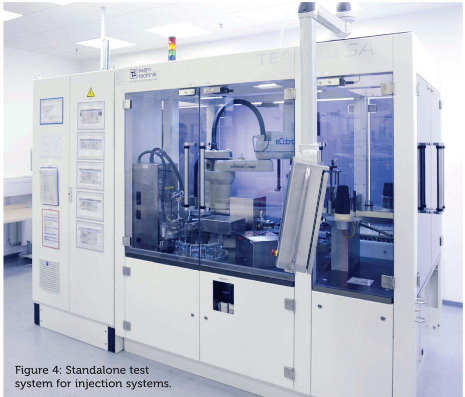
Figure 4: Standalone test system for injection systems.
