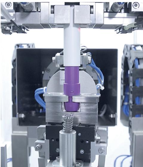
Figure 5: Torque measurement.
