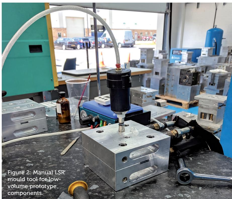
Figure 2: Manual LSR mould tool for low-volume prototype components.
