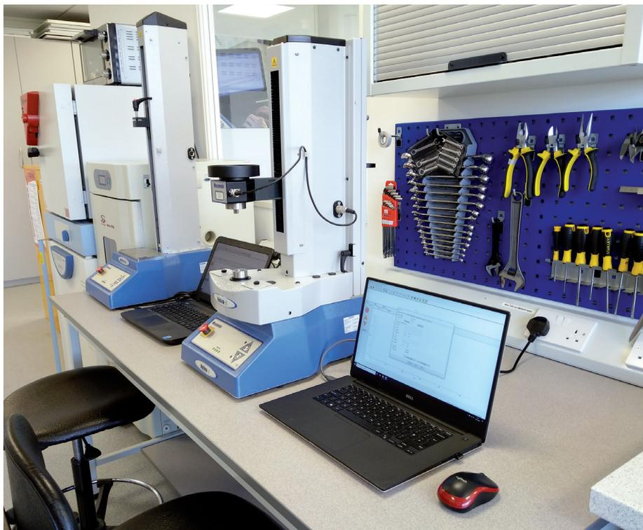
Figure 5: Mecmesin (Horsham, UK) force and torque testers.
