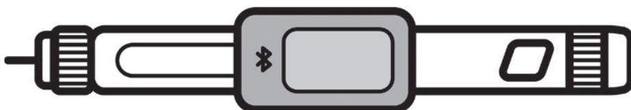
Figure 5: Specialised add-on for disposable pen injector, enabling key parameters detection to count administered doses accurately.
