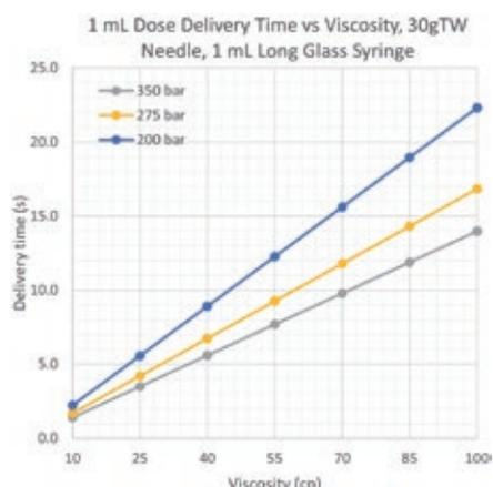
Figure 4: Small needle gauge delivery model data.
