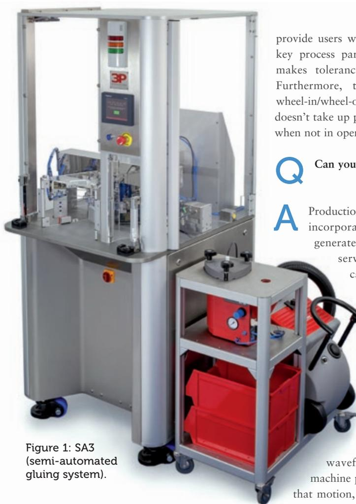
Figure 1: SA3 (semi-automated gluing system).
