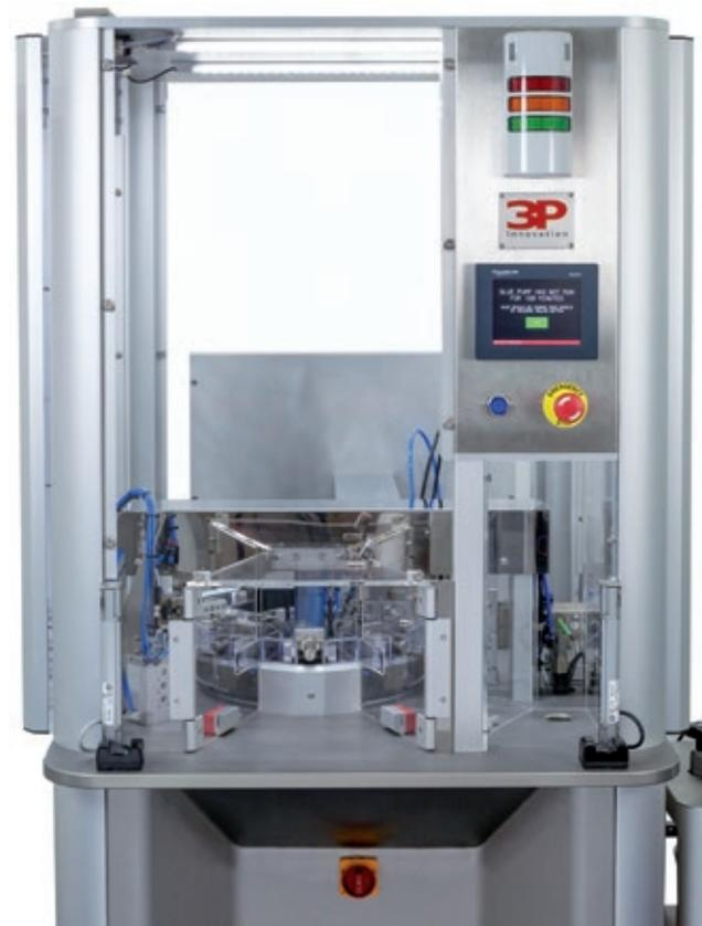
Plus, as you'd expect from a medtech automation supplier, it's fully GMP compliant with a validation pack and control system that's suitable for a 21 CFR 11-based electronic record system. With its engineering expertise, 3P offers a custom build service to cater for specific customer requirements, should they not fit within the normal operating envelope of the system.
