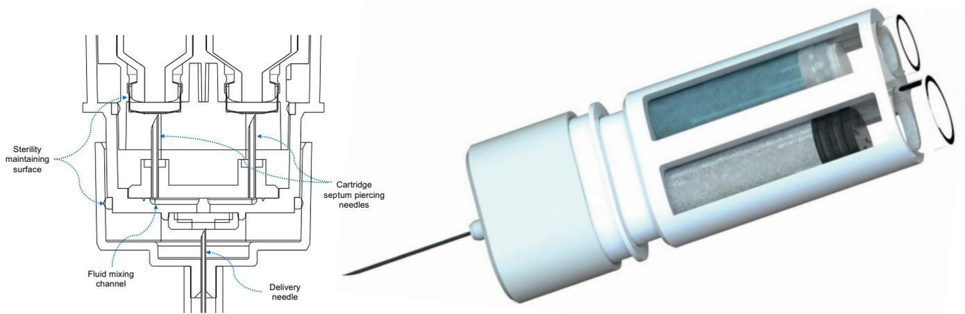
Figure 1: On the left, a cut-away schematic of Windgap's proprietary mixing and delivery hub. On the right, the novel side-by-side configuration of standard, single-chamber cartridges.
