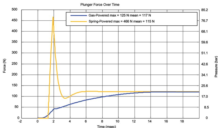
Figure 6: Force and pressure comparison between gas- and spring-powered autoinjectors.
