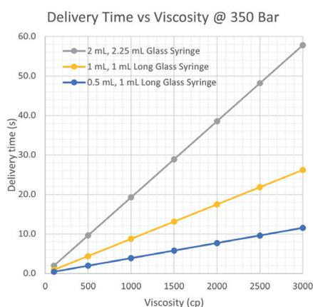
Figure 3: Ultra-high viscosity delivery time model data.
