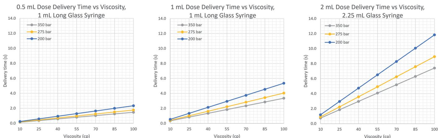
Figure 2: Dose delivery time versus viscosity model data.
