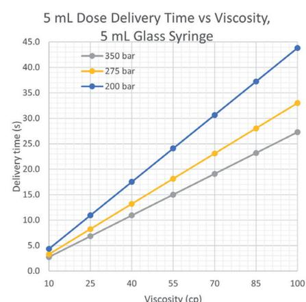
Figure 5: High-volume dose delivery model data.
