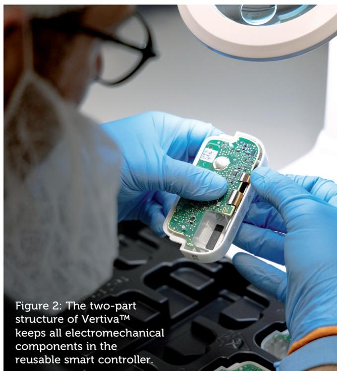
Figure 2: The two-part structure of Vertiva™ keeps all electromechanical components in the reusable smart controller.
