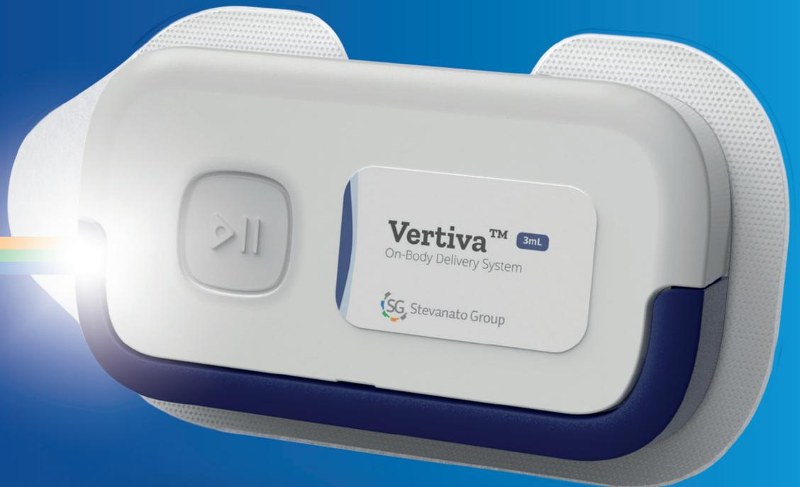
Composed of a single-use pod with **pre-filled and pre-loaded** cartridge and a multi-use, smart controller, Vertiva™ can deliver micro-precision basal doses and full-content bolus injections, resulting in a highly flexible and customizable platform **suitable for a wide range of therapies.**
