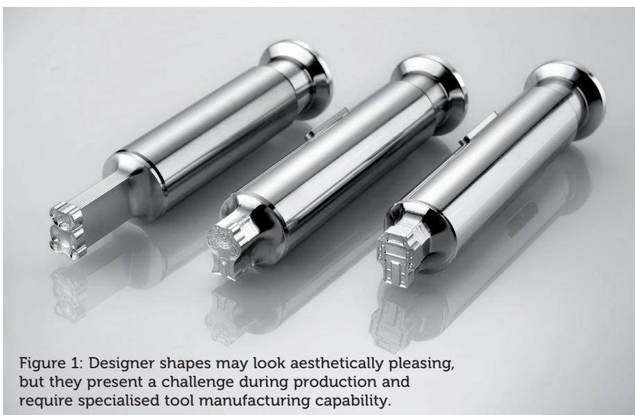
Figure 1: Designer shapes may look aesthetically pleasing, but they present a challenge during production and require specialised tool manufacturing capability.
