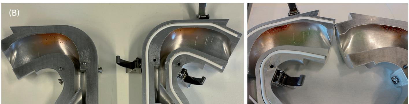
Figure 2: Deposition study of 0.5% fluorescein in 0.9% saline formulation using a next-generation impactor was performed with an airflow rate of 20 L/min. (A) Deposition based on emitted mass; (B) Deposition in an Alberta Idealized Throat (left: lung inhaler; right: larynx inhaler).
