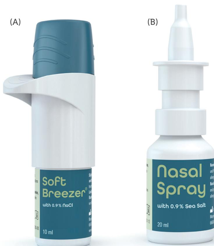
**Figure 3:** A: The SoftBreezer and the SoftBreezer Larynx are designed in line with a standard portable-inhaler design. They are propellant free and preservative free and generate a fine nebulisation. Exact dosages are generated and the actuation time dependent on the pore size is 1–3 s. B: The nasal spray for the soft mist generation embeds the spray nozzle unit inside the spray nozzle of a standard metered-dose nasal spray.
