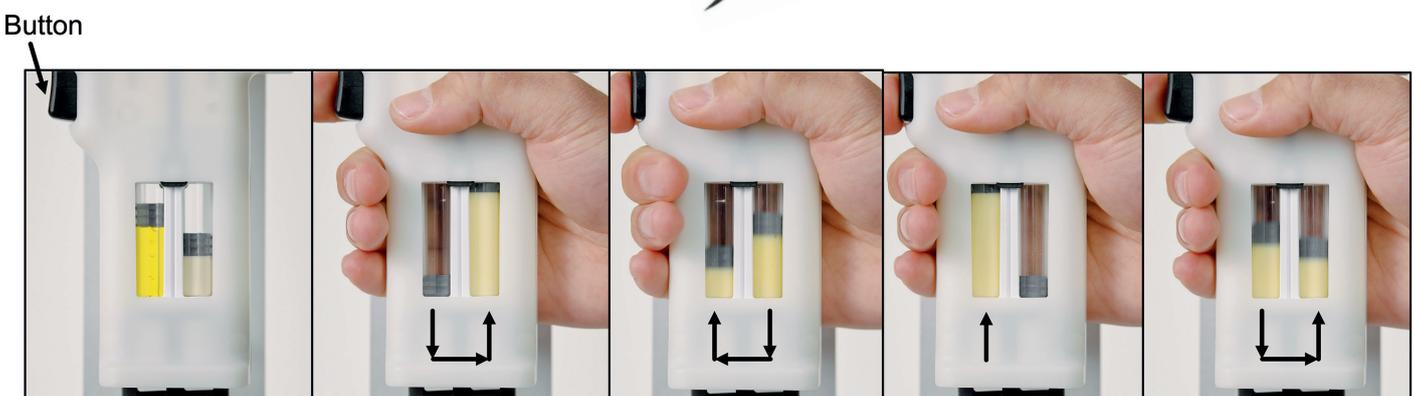
Figure 3: Demonstration of Windgap's reciprocating autoinjector mixing a cyanide antidote drug product currently under development. Arrows indicate alternating fluid flow in the PDC between cartridges.
