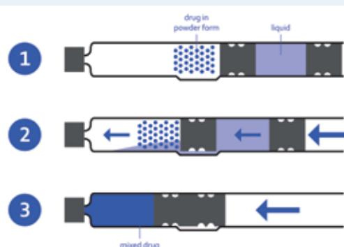
Figure 2: Dual-chamber cartridge.
