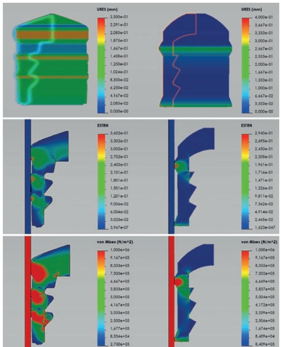
Figure 2: Simulating and comparing strain and stress profiles of unsilicised lubrigone<sub>3</sub> plungers and a coated butyl rubber plunger in glass, in the conversion from dynamic state to motion by combining a nonlinear simulation of hyperelastic using Mooney-Rivlin and a linear elastic deformation using Mohr-Coulomb. Left: Butyl rubber plunger stopper; Right: lubrigone<sub>3</sub> plunger stopper; Top: Deformation of plunger stopper; Mid: Maximum strain; Bottom: Maximum stress.
