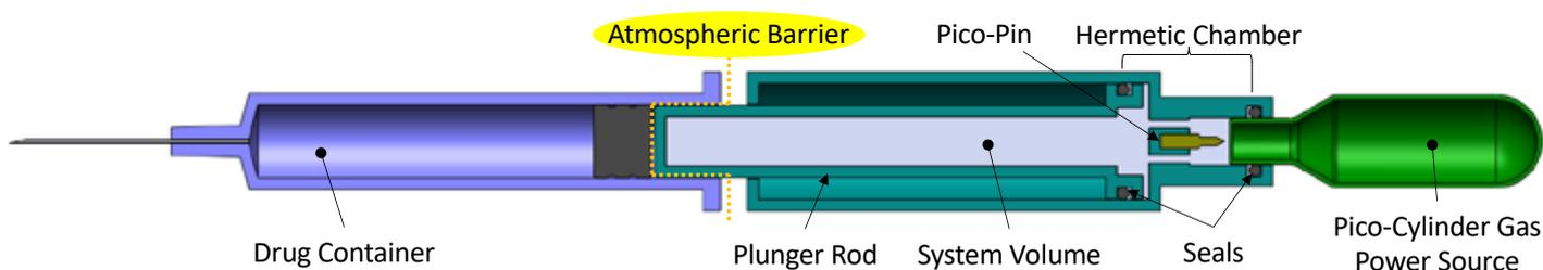
Figure 2: Gas pressure isolation from primary drug container.
