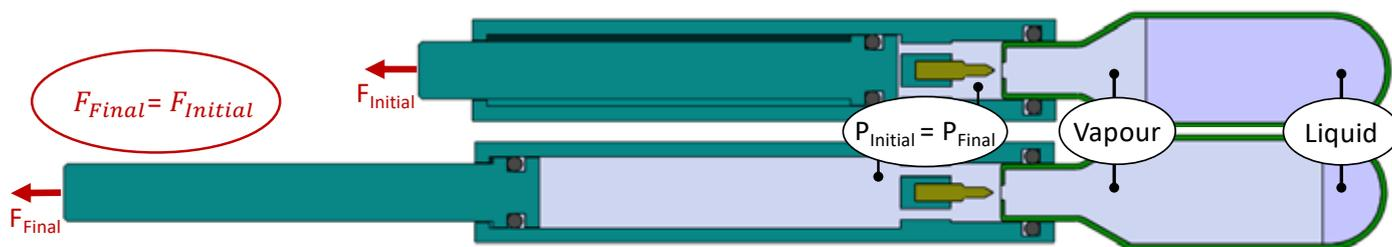
Figure 5: Dual-phase gases provide a constant pressure at a set temperature resulting in a constant force profile.
