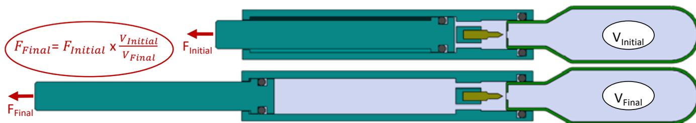
Figure 6: Force drop over stroke due to increase in internal volume as plunger deploys.
