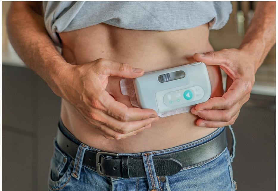
Figure 3: Simulated use of Symbioze® on-body injector prototype.
