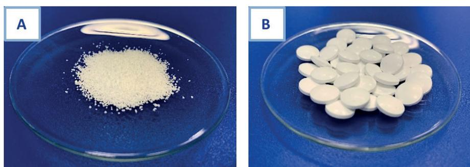
Figure 3. Granulated powder (A) used to produce lipid nanoparticle-based tablets (B).
