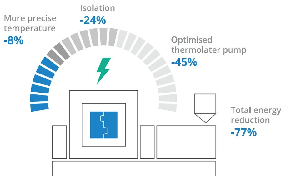
Figure 2: In the optimised test, an energy reduction of 77% was achieved.
