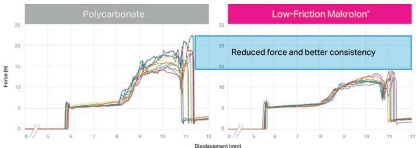
Figure 3: Forces versus displacement for button fire with polycarbonate (left) and medical-grade low-friction Makrolon (right).
