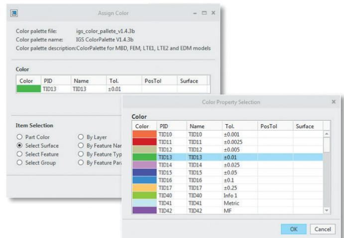
Figure 2: Colour-coding system.
