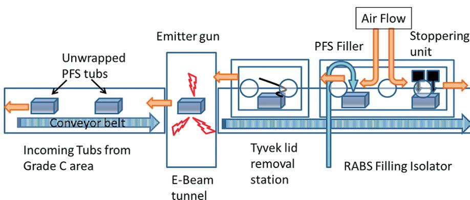
Figure 3: A schematic of an E-beam/RABS fill-finish system.
