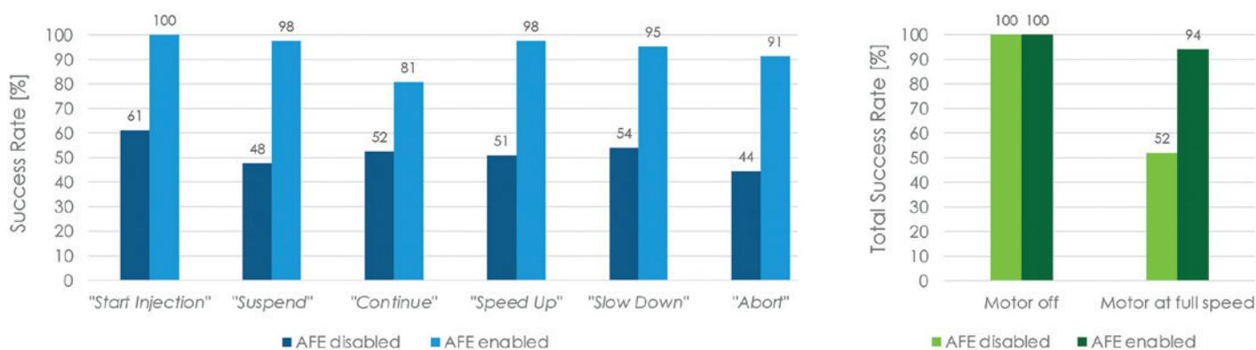
Figure 4: Keywords recognition accuracy. Test performed on 20 US-native subjects (ten male, ten female) with autoinjector's motor operated at full speed (noise level 68 dB(A)).
