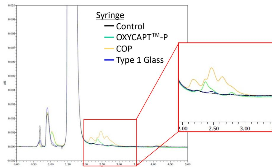
Figure 7: Impurities recognised on a chromatogram of syringes.
