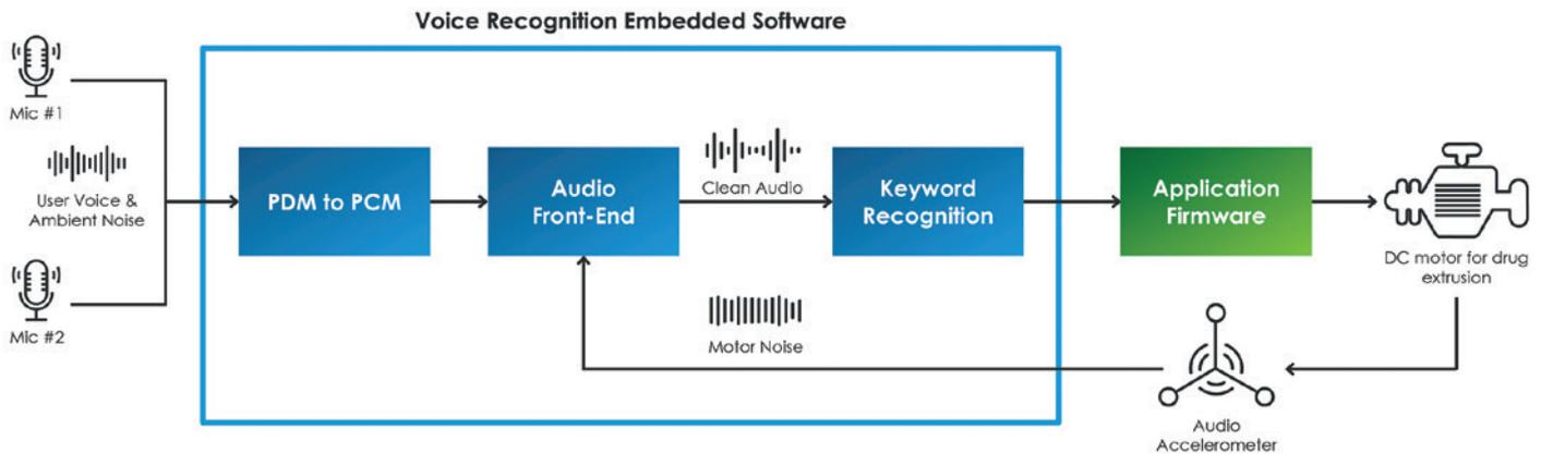
Figure 2: Block diagram of the voice-processing system.
