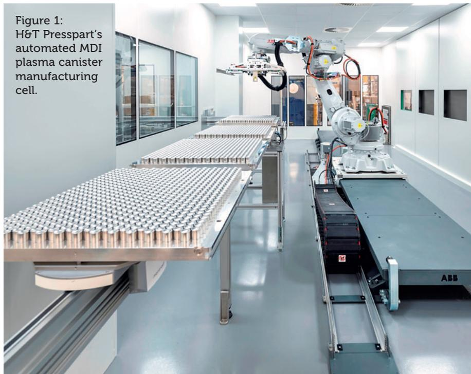
Figure 1: H&T Presspart's automated MDI plasma canister manufacturing cell.
