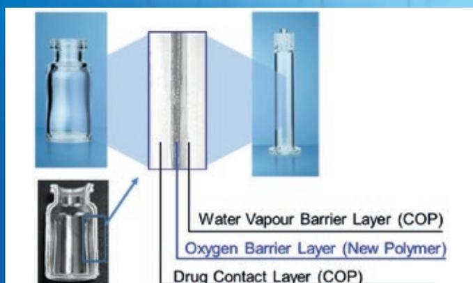
Figure 2: Multilayer structure of OXYCAPT.
