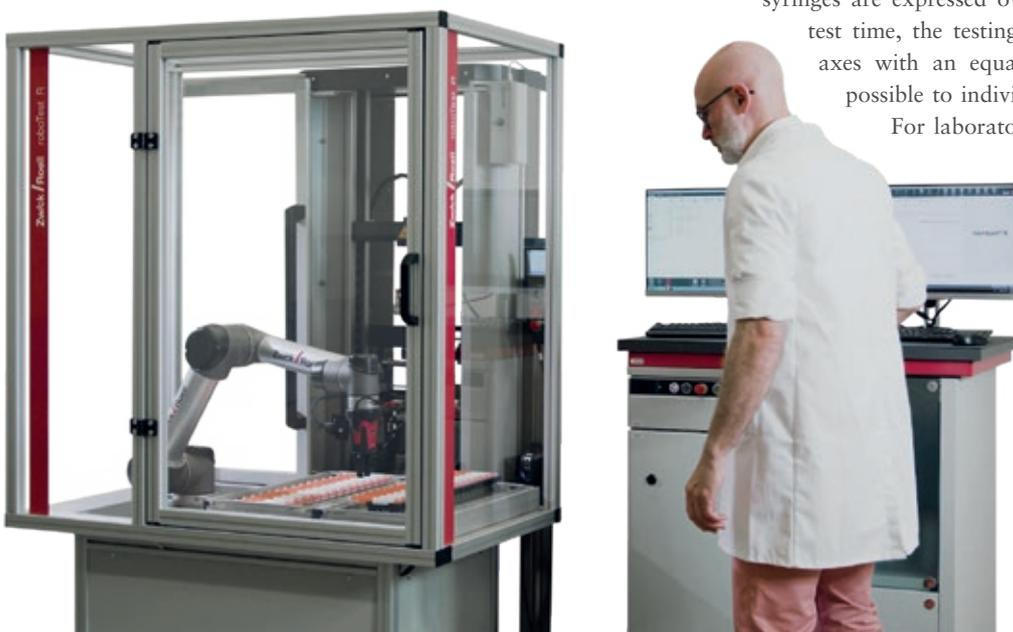
Figure 1: Fully automated testing systems for autoinjectors.
