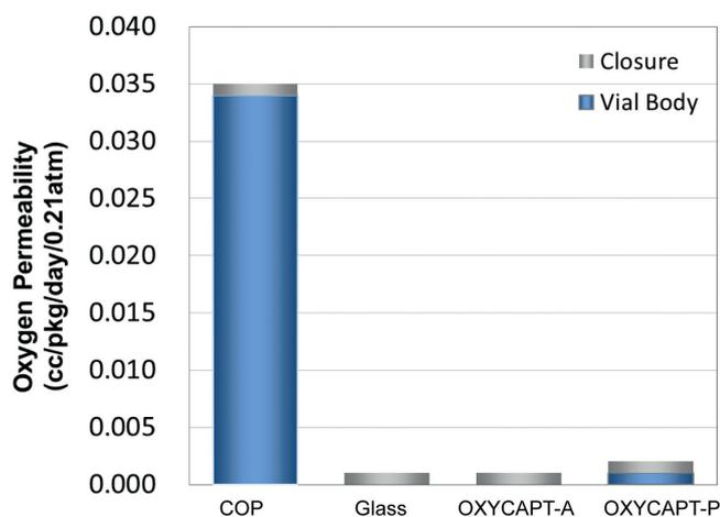
Figure 3: Comparison of the oxygen barrier properties of glass, COP, OXYCAPT-A and OXYCAPT-P.
