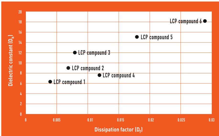
Figure 4:  $D_k/D_f$  values for high  $D_k$  Zenite LCPs, measured via International Electrotechnical Commission (IEC) 61189-2-721 method at 2 GHz.
