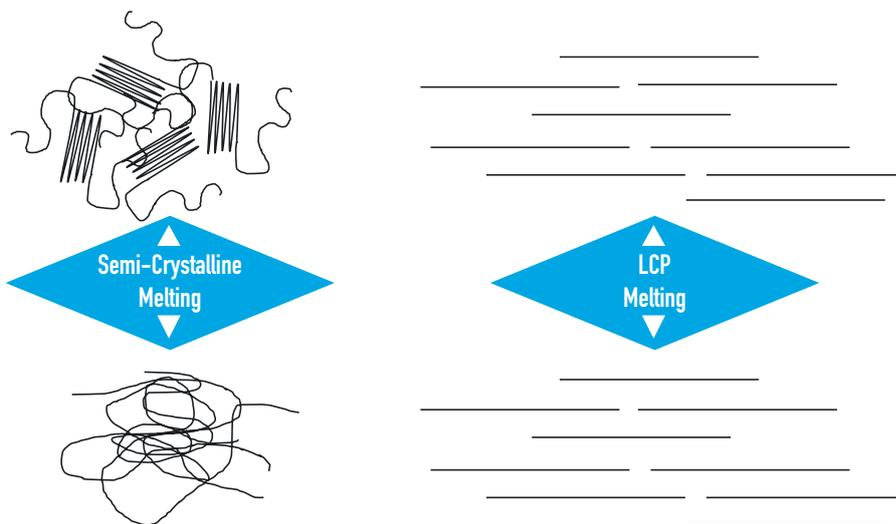
Figure 3: The unique morphology of LCP leads to rapid solidification and short moulding cycles.
