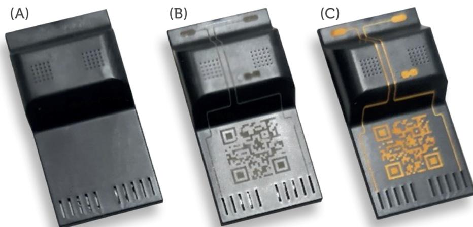
Figure 6: Example of laser direct structuring of circuit interconnects.
