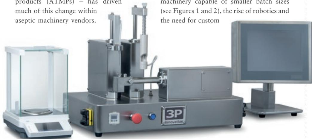
Figure 1: Ultra-low scale fill-finish (3P's F2V).
