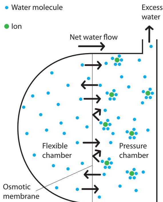
Figure 2: Schematic representation of the osmotic process in the Subcject wearable injector.
