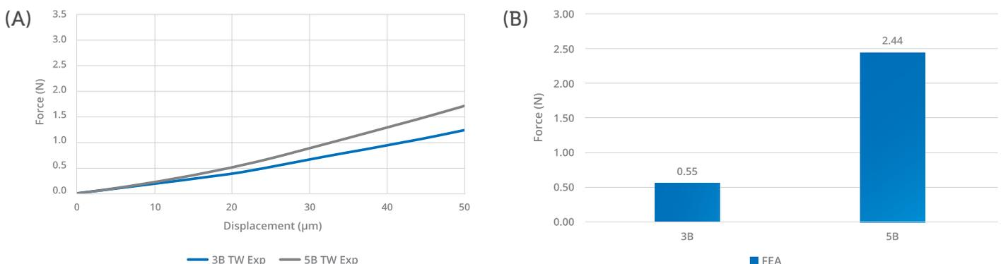
Figure 2: The finite element analysis confirmed a significantly lower hooked needle propensity for the five-bevel needle tip design compared with the three-bevel needle tip design. The trend (A) and external load (B) required to generate a hooked needle at 50 μm is significantly higher – approximately five times – for the five-bevel needle tip design than with the three-bevel needle tip design.
