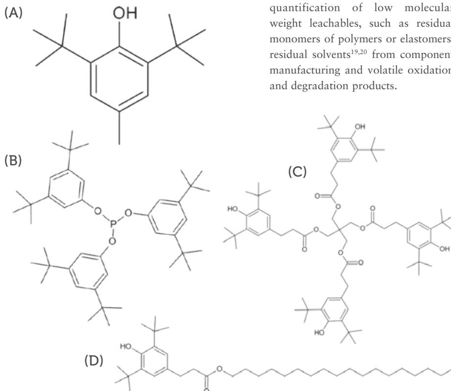
Figure 3: Typical antioxidants used as polymer additives. (A) BHT, (B) Irganox 168, (C) Irganox 1010 and (D) Irganox 1076.
