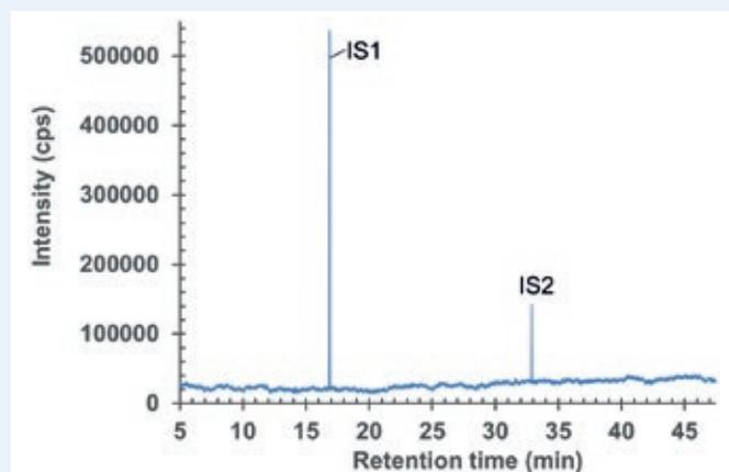
Figure 6: GC-MS chromatogram of polymer syringe barrel after extraction in water (pH 5.2).
