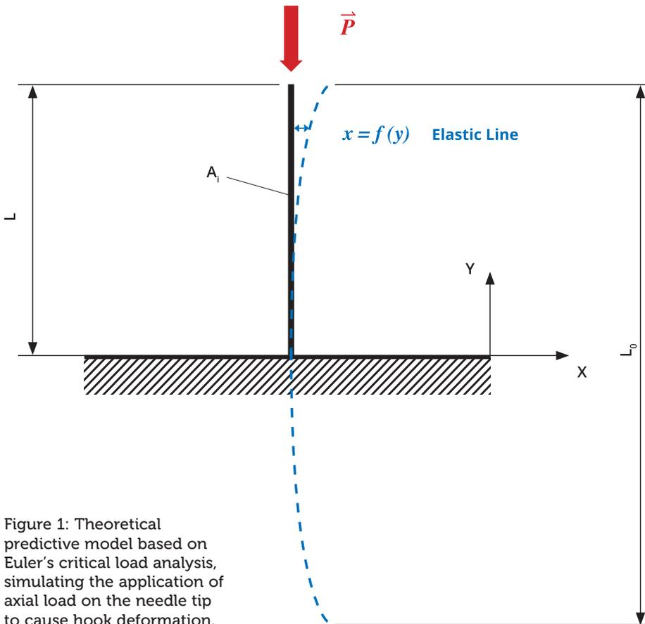
Figure 1: Theoretical predictive model based on Euler's critical load analysis, simulating the application of axial load on the needle tip to cause hook deformation.
