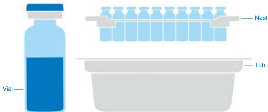
Figure 1: Components of a sterile ready-to-use packaging solution.
