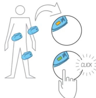
4. EJECT & DISPOSE OF RESERVOIR
