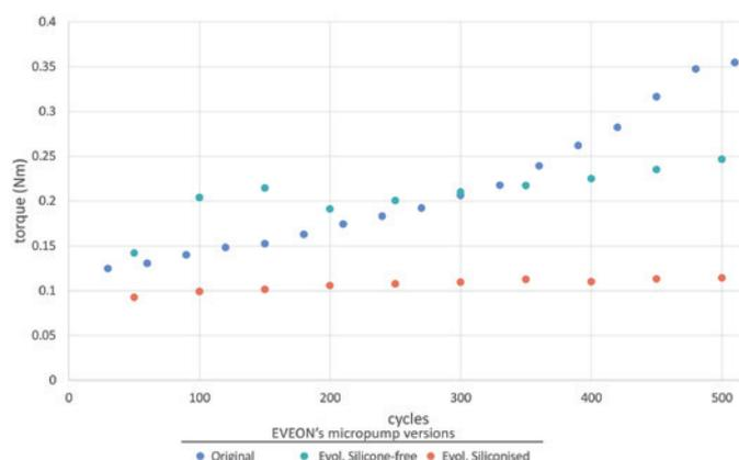
Figure 2: Torque as a function of number of cycles at 80 rotations per minute for three different versions of EVEON's proprietary micropump: original, evolution (silicone-free) and evolution (siliconised).
