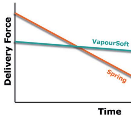
Figure 1: Change in force applied to a syringe in an autoinjector with a standard spring (red) and a liquefied gas-powered system such as Bespak's VapourSoft (blue).
