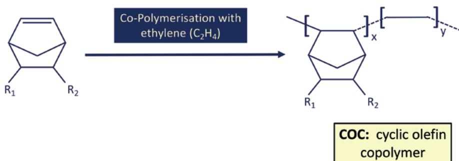
Figure 2: Structure and synthesis of a COP. Poly(norbornene-co-ethene) is represented where R1 and R2 are hydrogen.
