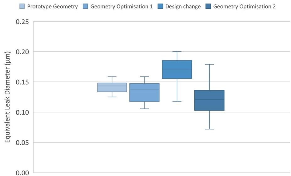
Figure 4: Boxplot showing an example of CCI performance optimisation using hydrogen leak testing. Tests performed at room temperature ( $23\pm 5$ ) °C and ( $50\pm 25$ ) % relative humidity (left to right: Plots 1-3  $n\geq 10$ , Plot 4  $n=30$ ).
