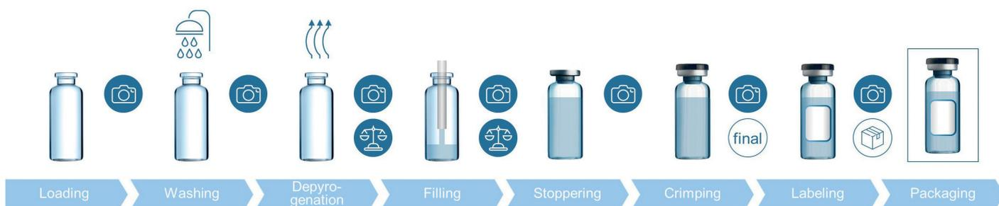
Figure 3: Laser-marked containers and cameras located at different positions on the filling line allow each individual item to be tracked throughout the fill-and-finish process.
