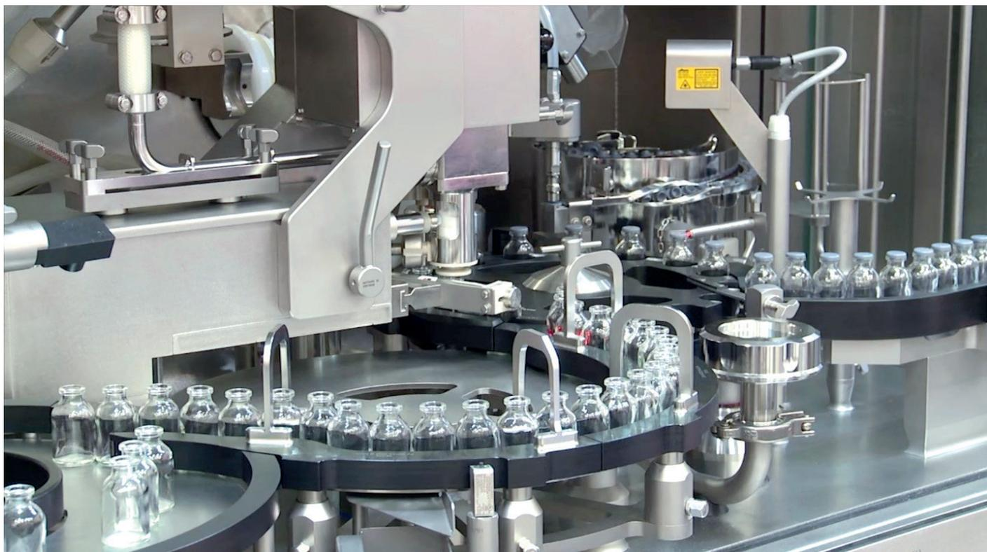
Figure 5: A modular, automated aseptic line at Evonik's Birmingham (AL, US) site for the filling of powders, liquids or suspensions into vials.
