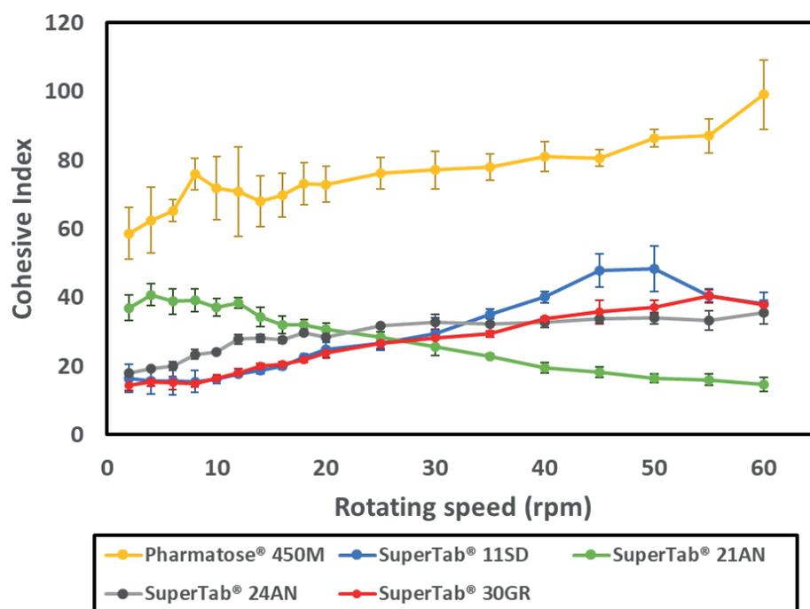
Figure 4: Cohesive index versus rotating drum speed. Shear-thickening behaviours are observed, except for powder SuperTab® 21AN, which exhibits strong shear-thinning behaviour.
