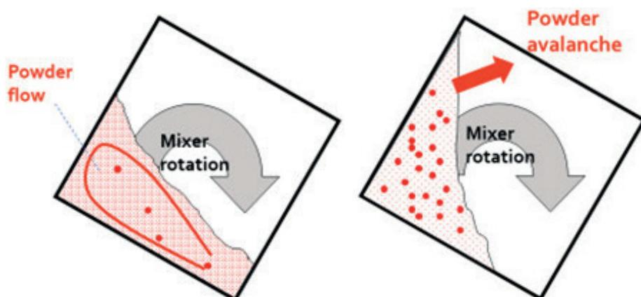
Figure 1: Free-flowing powders tend to set up a rolling motion inside the powder bed, resulting in ball milling of the API agglomerates. Poor-flowing powder tends to avalanche and results in less motion inside the powder bed and less ball milling of API agglomerates.
