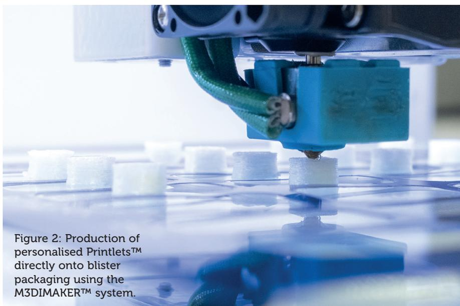
oral dosage forms using computer-aided design (CAD) software for the on-demand, layer-by-layer production of Printlets™ (3D printed tablets).<sup>2,3</sup>
