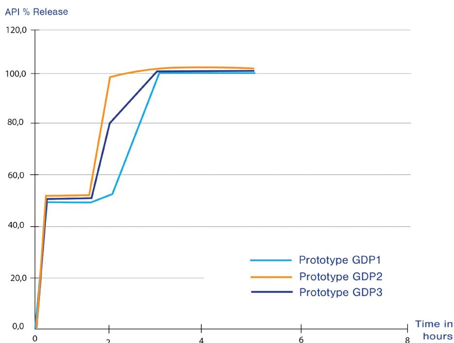
Figure 4: Dissolution profiles obtained for the different Geoclock® double pulse prototypes.
