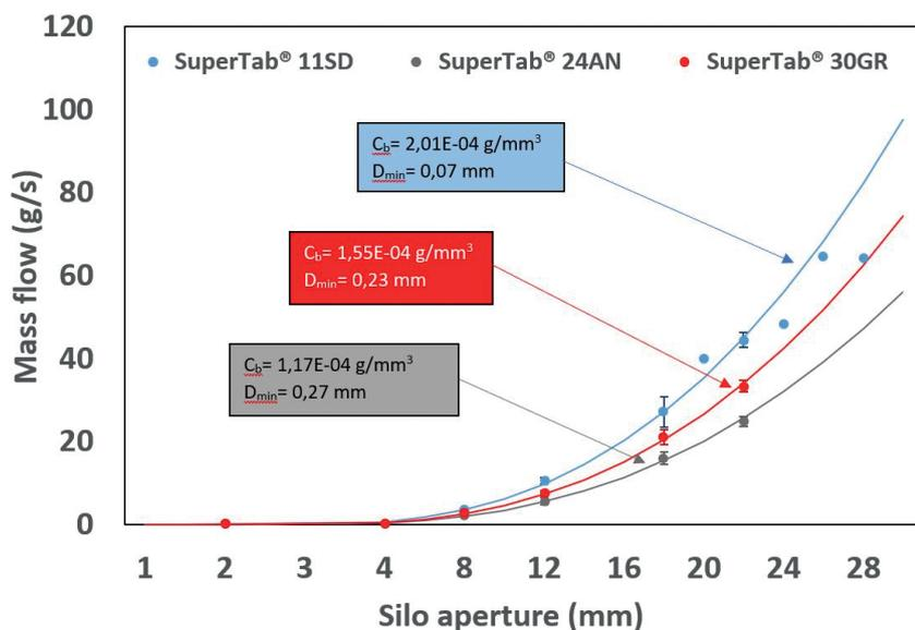
Figure 3: Mass flow rate versus aperture for powders.
