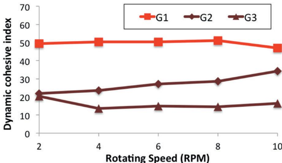
Figure 4: Dynamic cohesive index of the granules measured from the fluctuations of the flow in GranuDrum.
