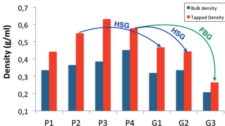
Figure 5: Bulk and tapped densities obtained with the automatic measurement instrument GranuPack.
