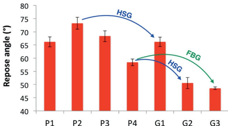
Figure 2: Repose angle measured with GranuHeap. The measurement is repeated three times to perform an average and the error bars correspond to the standard deviation.
