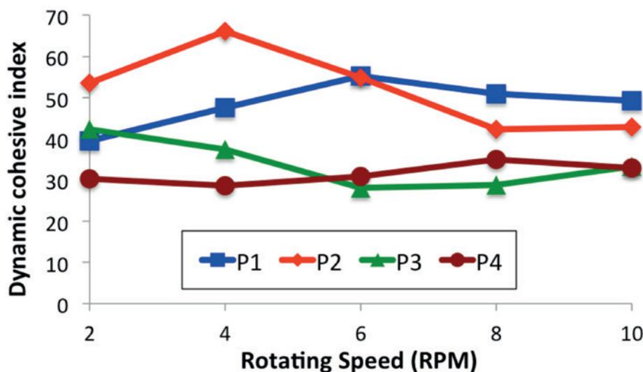
Figure 3: Dynamic cohesive index of the powders measured from the fluctuations of the flow in GranuDrum.
