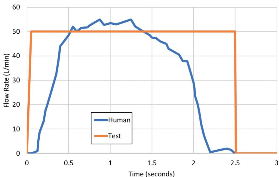
Figure 1: Differences between human and test flow profiles.
