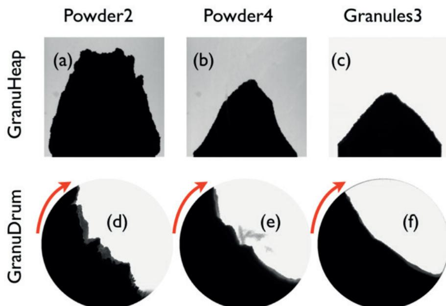
Figure 1: Typical pictures of heaps and of the flow inside the rotating drum with two powders (P2 and P4) and with G3 granules.
