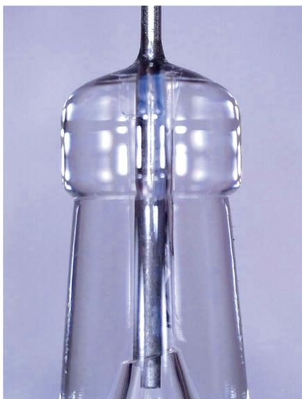
Figure 1: UV-cured adhesive bonding needle to syringe.
