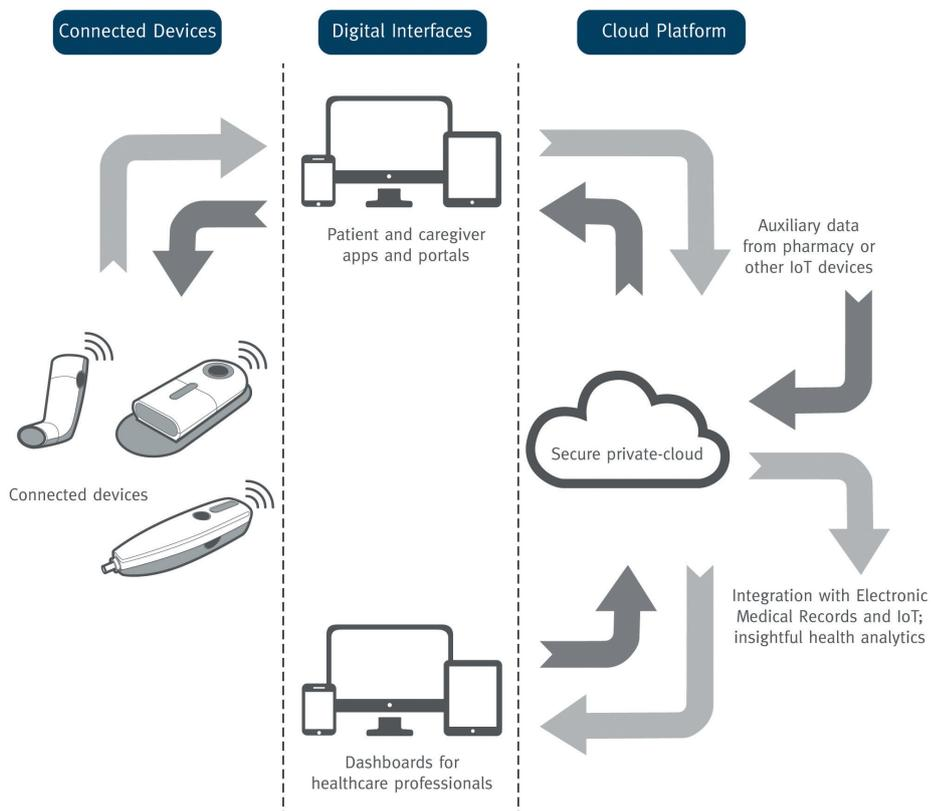
Figure 3: The three primary components of a connected health ecosystem.
