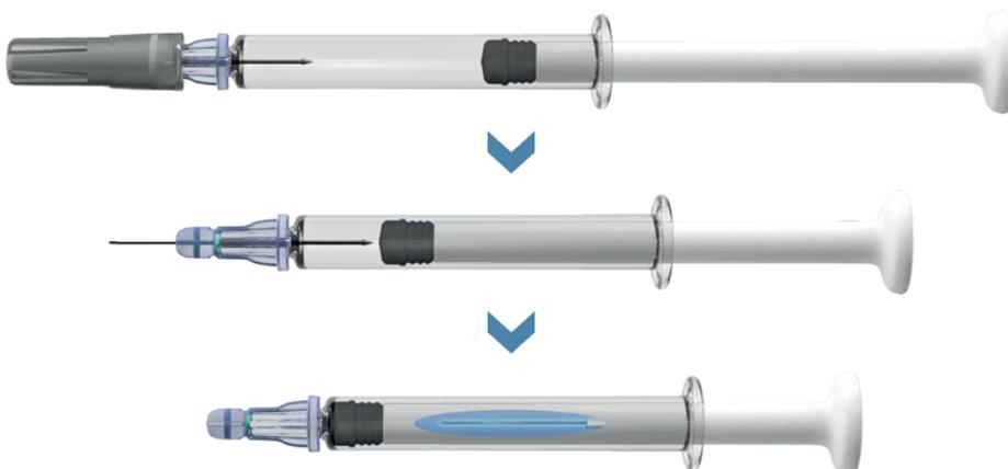
Figure 2: With the Credence Companion®, the user performs the injection, receives end-of-dose cues and then the needle automatically retracts into the syringe, preventing re-use.
