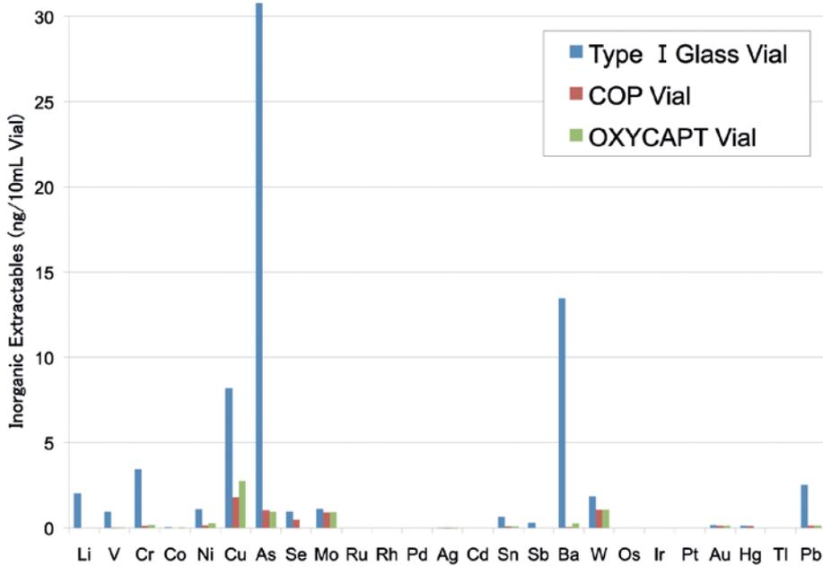
Figure 5: Graph comparing inorganic extractables levels from OXYCAPT™ with those from COP and glass.
