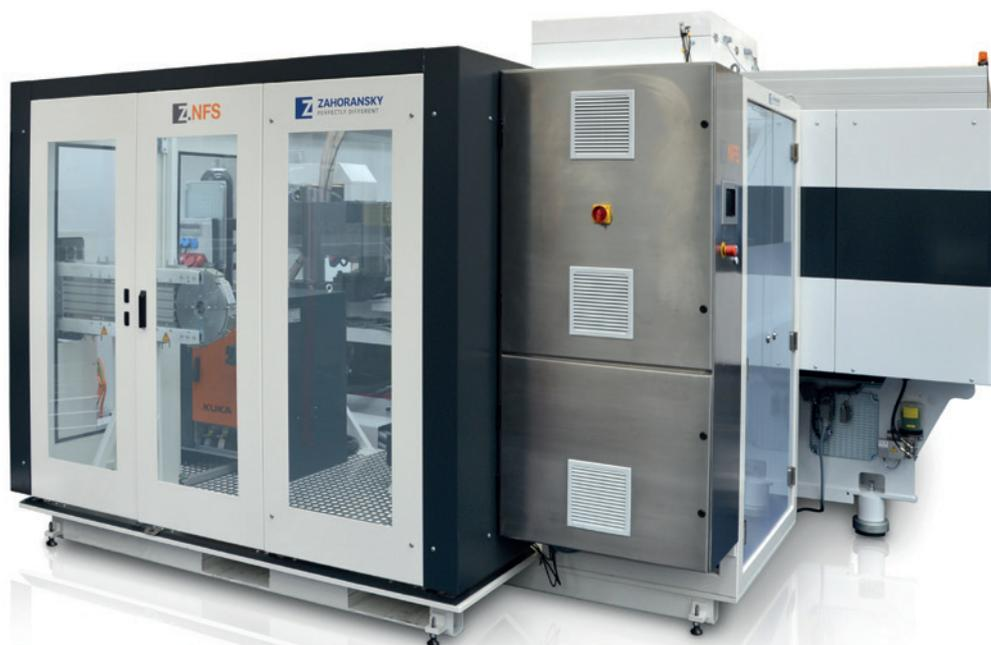
Figure 1: The Z.BLIZZARD produces ready-to-fill PFS from COC/COP polymer with a very long autonomy time.
