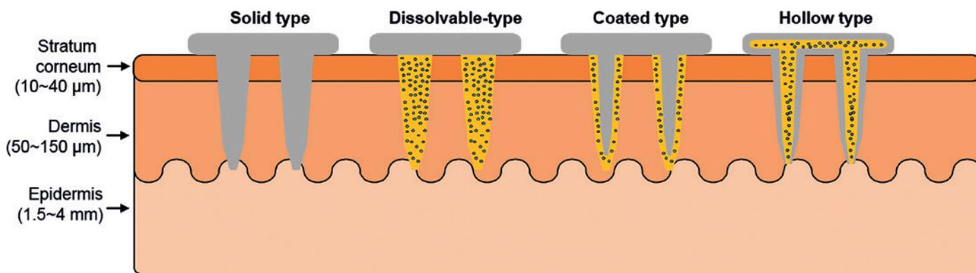
Figure 1: Schematic illustration of various needle forms.
