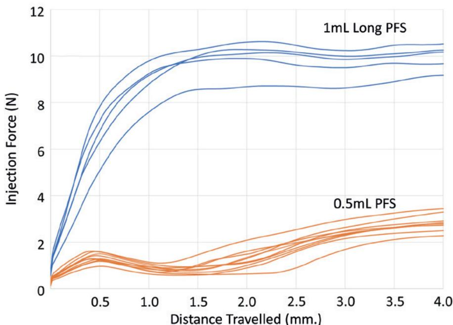
Figure 4: Force with 0.5 mL PFS (orange) and 1 mL “long” PFS (blue), both with baked-on silicone when injecting water with 30-gauge ½” needle.
