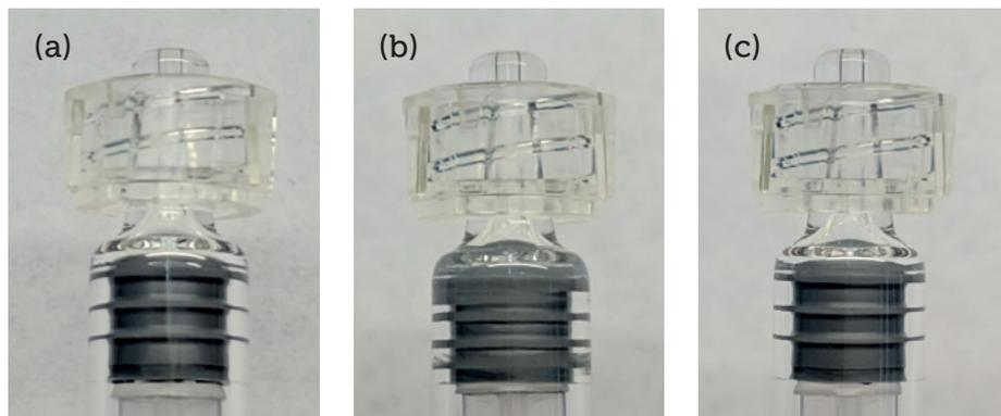
Figure 2: User variation in end-of-injection position of plunger stopper: just bottomed out (a), forced into the shoulder region (b), and retracted having been forced into the shoulder region (c).
