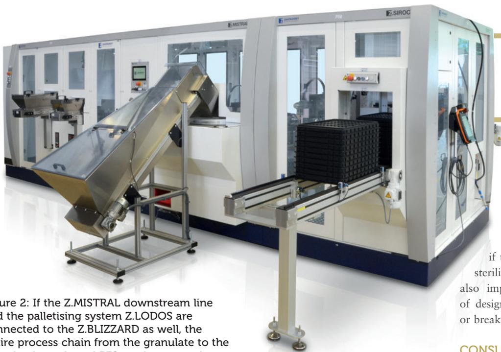
Figure 2: If the Z.MISTRAL downstream line and the palletising system Z.LODOS are connected to the Z.BLIZZARD as well, the entire process chain from the granulate to the completely packaged PFS can be covered.
