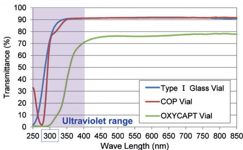
Figure 4: Graph comparing UV transmission properties of OXYCAPT™ with COP and glass.
