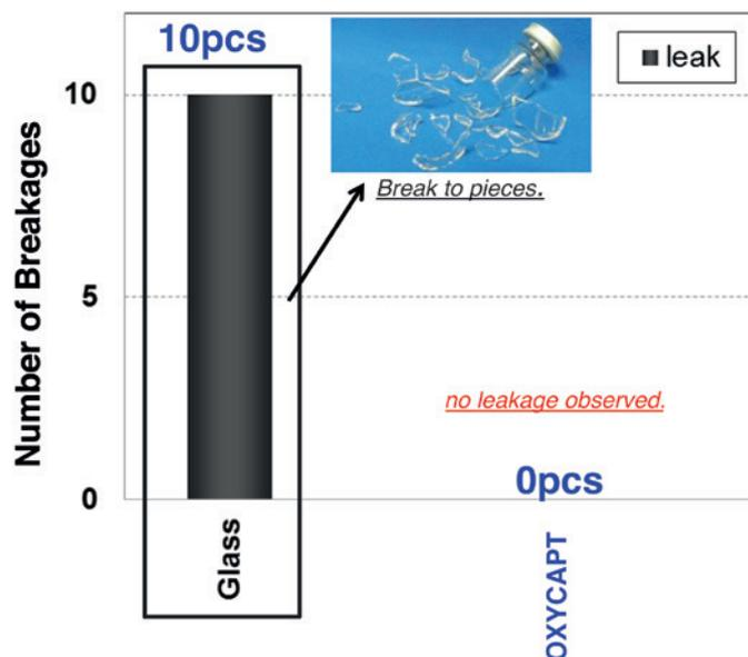
Figure 7: Zero OXYCAPT™ breakages during drop test, compared with 100% breakage with glass.
