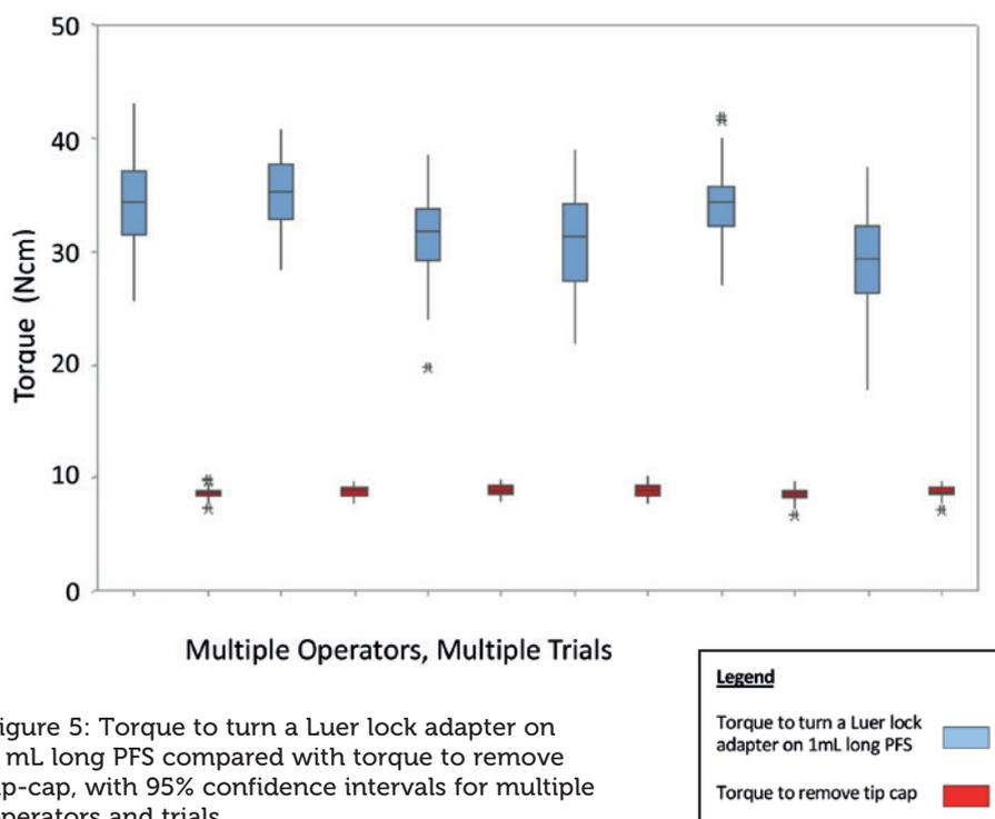
Figure 5: Torque to turn a Luer lock adapter on 1 mL long PFS compared with torque to remove tip-cap, with 95% confidence intervals for multiple operators and trials.
