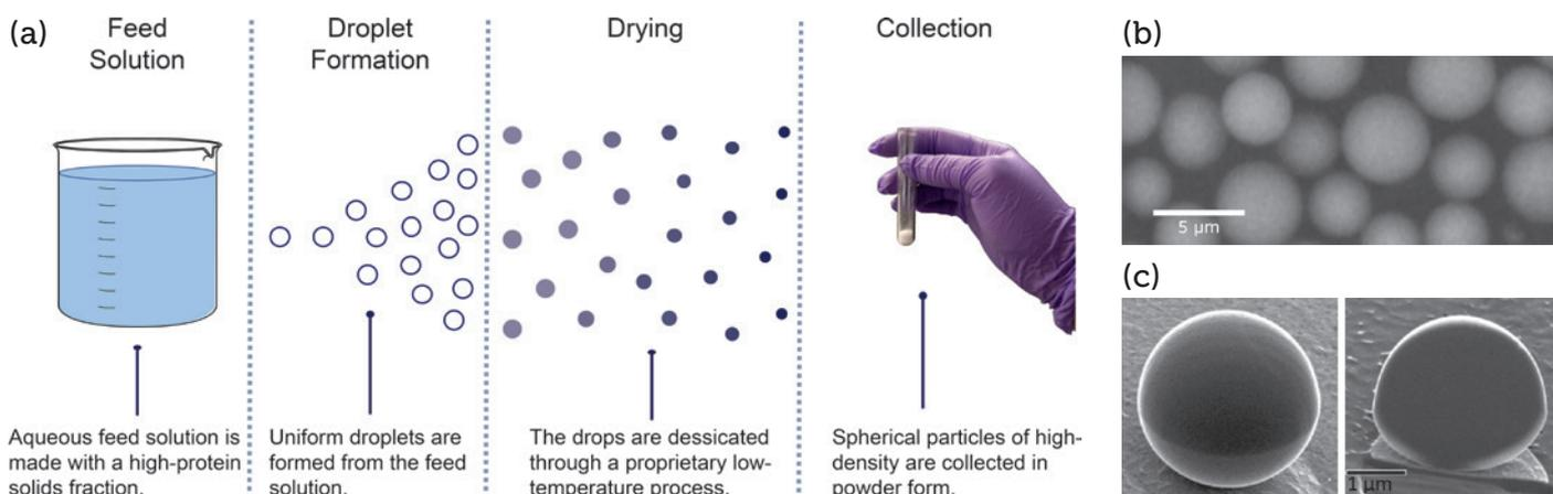
Figure 1: Elektroject™ microparticle production process (a), microparticles (b), and a cross section of a single microparticle demonstrating non-porous morphology (c).
