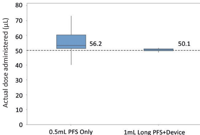
Figure 3: Boxplot with 95% CI of ophthalmologists (n=21) attempting to inject 50 µL with a 0.5mL PFS only and device + 1 mL “long” PFS (n=100) in a lab setting.
