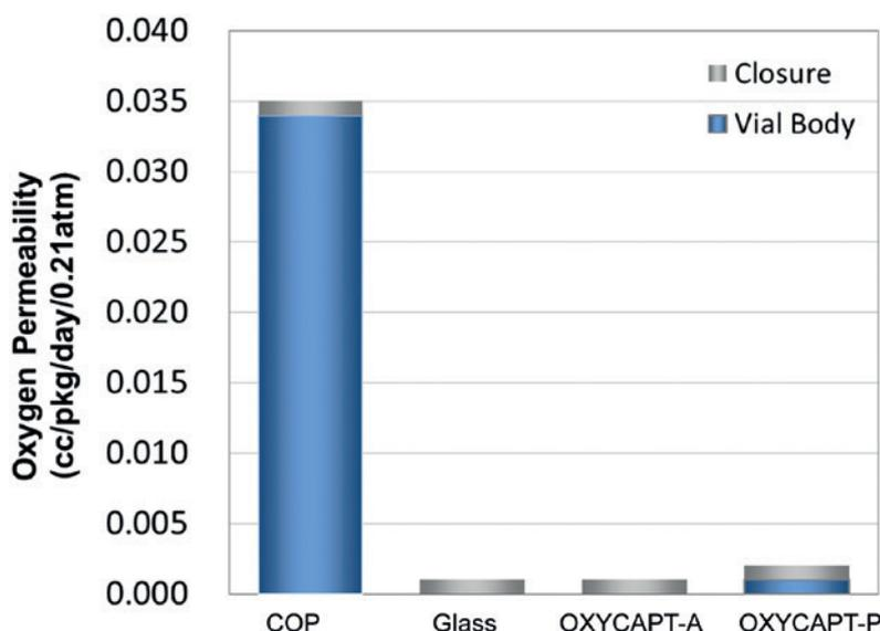
Figure 3: Graph comparing oxygen permeation properties of OXYCAPT™ with COP and glass.
