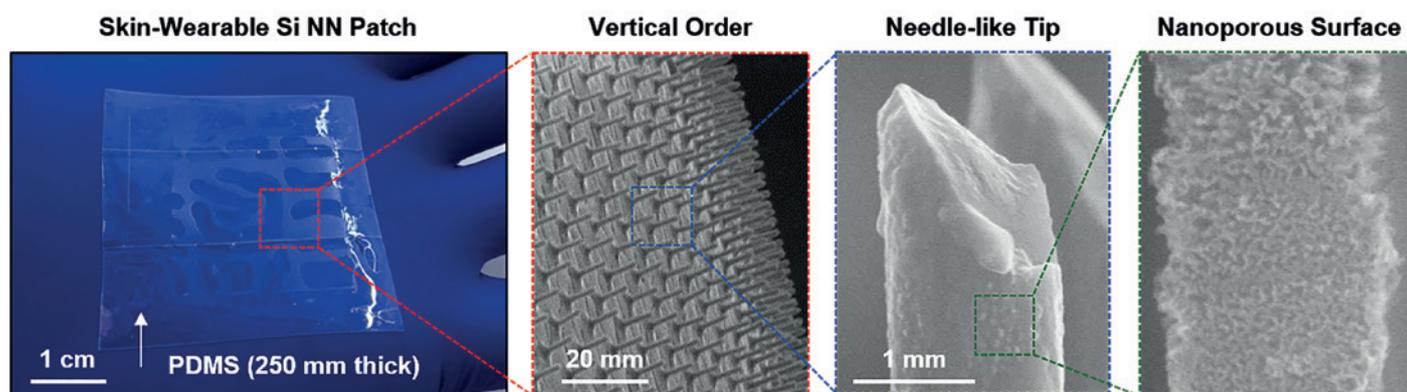
Figure 2: Photograph of a representative Si NN-patch (left) and magnified images of the tips and the nanoporous surface.
