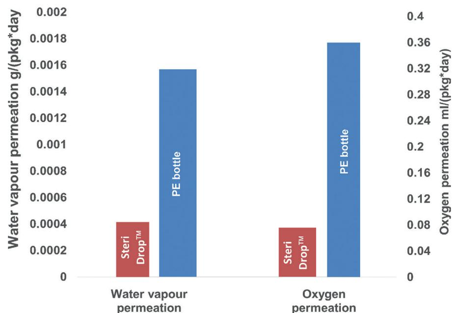
Figure 3: Water vapour and oxygen permeation results for polyethylene bottles and SteriDrop™ tubes.
