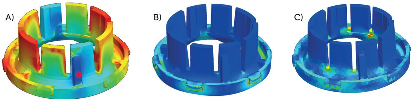
Figure 2: Engineering analysis in product development. (A) mould flow analysis during part fill; (B) von mises stress analysis during assembly; (C) the engineering strain analysis during cap removal.
