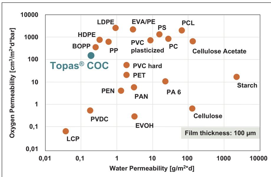
Figure 1: Topas barrier properties (relative humidity: 85%, temperature: 23°C)
