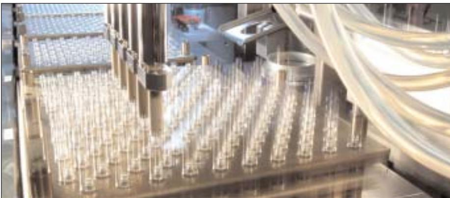
**Figure 4:** Filling of dual chamber cartridges
