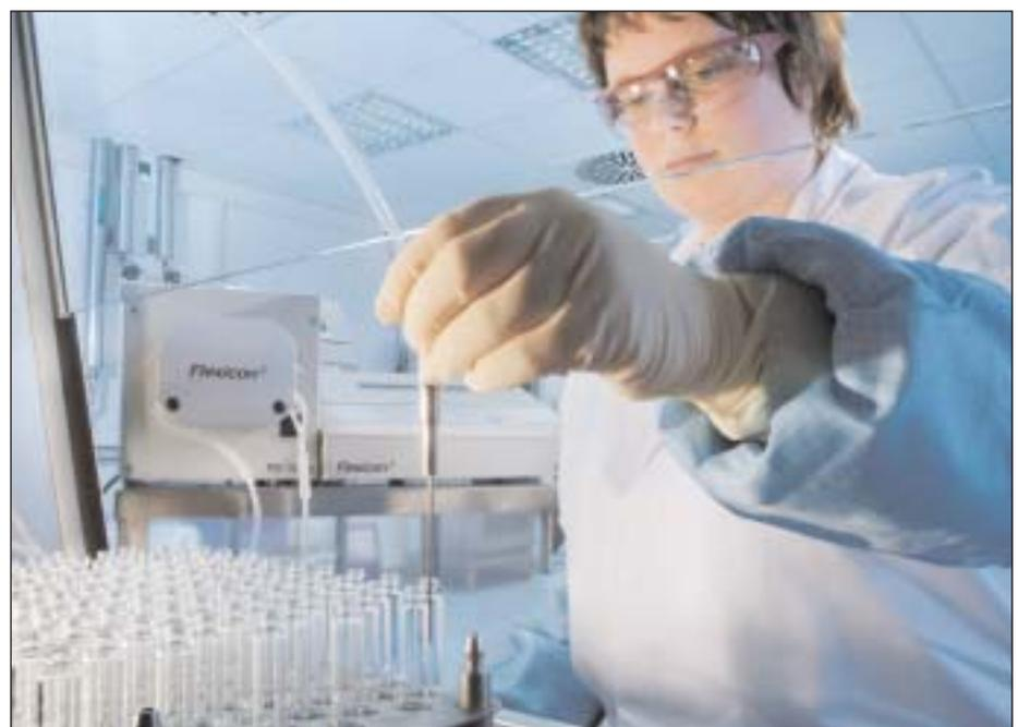
Figure 2: Filling operation via peristaltic pump
