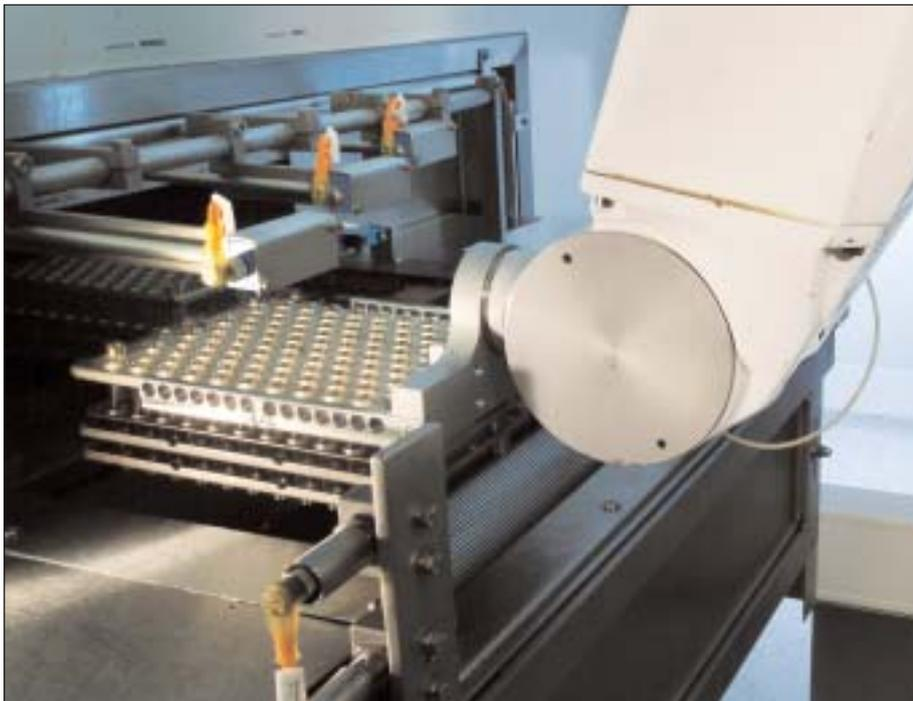
Figure 1: Automated heat tunnel unloading
