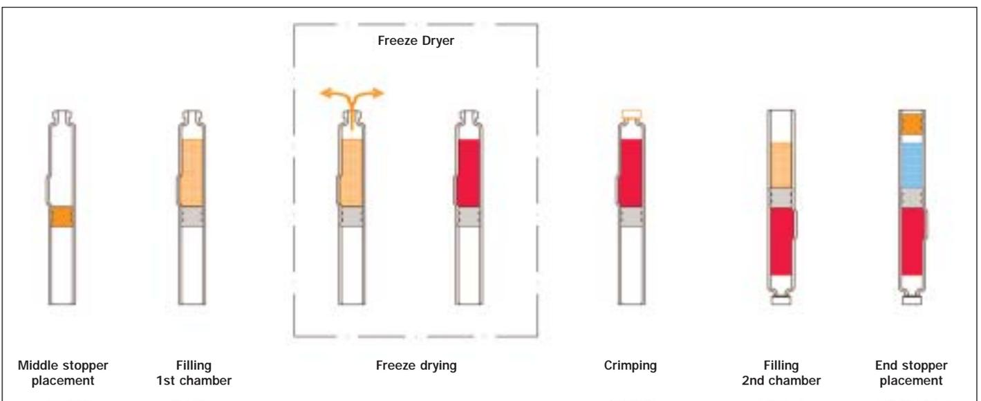
**Figure 5:** Steps involved in filling dual-chamber syringe
