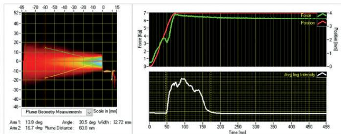
Figure 4: Comparison across plume geometry measurements between an unopened valve, partially opened and a fully opened valve.
