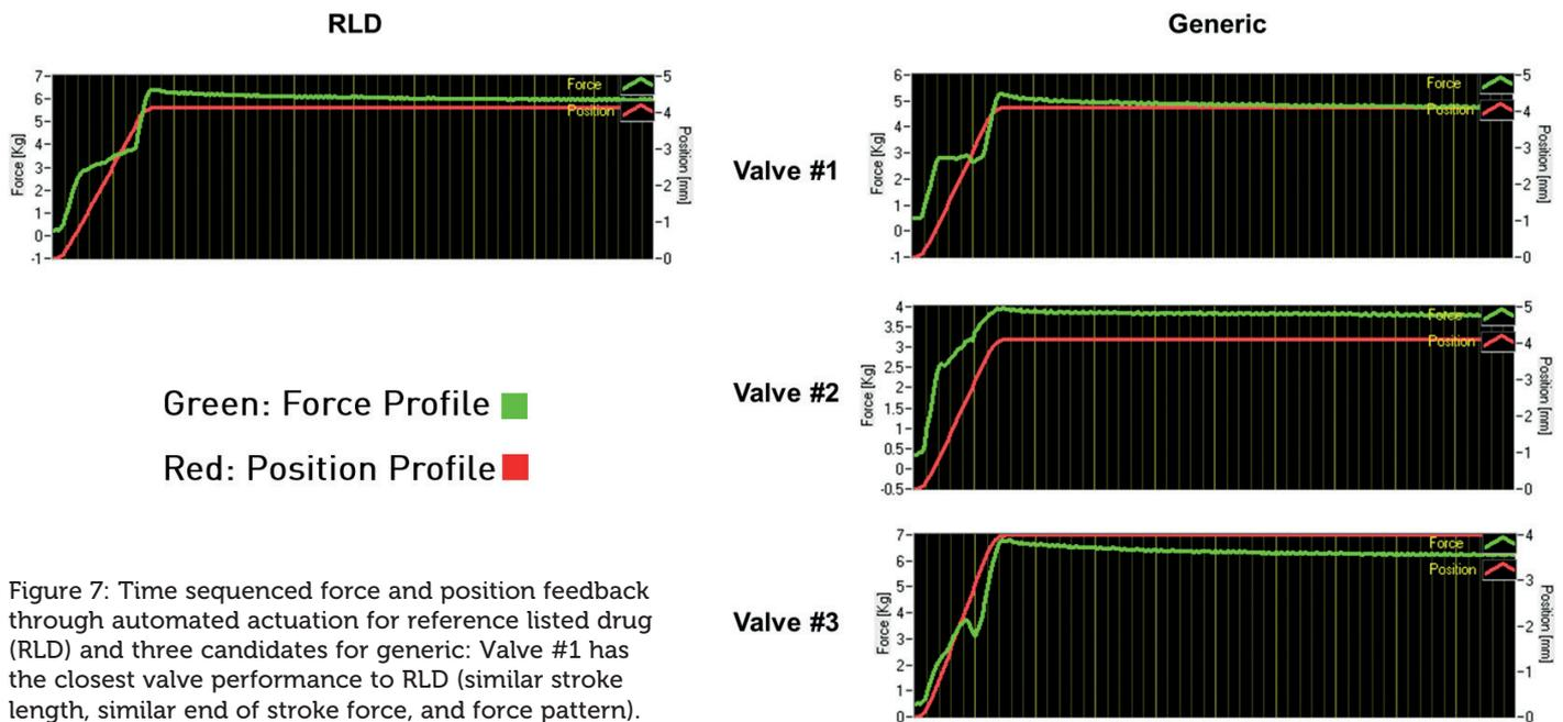
Figure 7: Time sequenced force and position feedback through automated actuation for reference listed drug (RLD) and three candidates for generic: Valve #1 has the closest valve performance to RLD (similar stroke length, similar end of stroke force, and force pattern).
