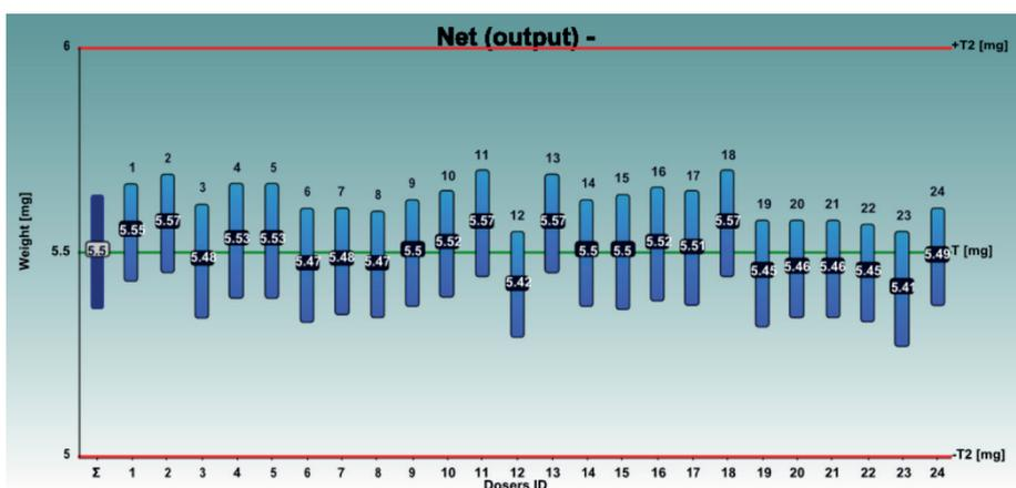
Figure 5: Respirose SV003 + 4% Lactose microfine, behaviour of the 24 dosators on Adapta.
