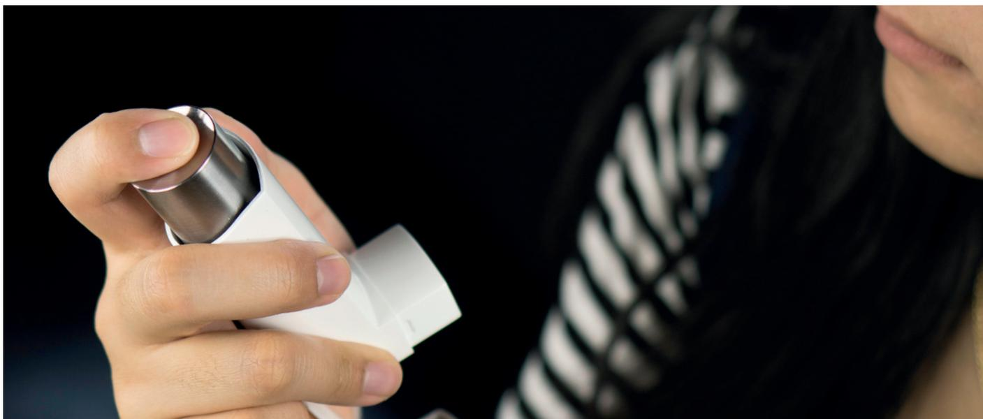
Figure 1: MDI training device designed to replicate an actual MDI's form factor and operation while providing the user with multisensory feedback.
