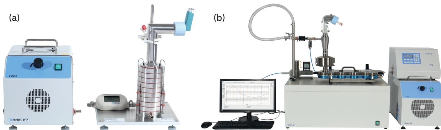
Figure 2: Test set-ups for APSD measurement depend on the purpose of testing such as: a simple ACI set-up for QC for MDIs (a), or an NGI set up for enhanced IVIVCs for DPIs (b).
