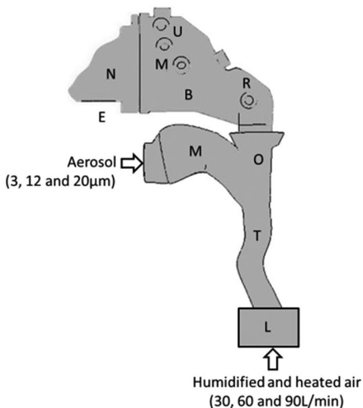
Figure 2: Experimental set up using the VCU upper airways model.
