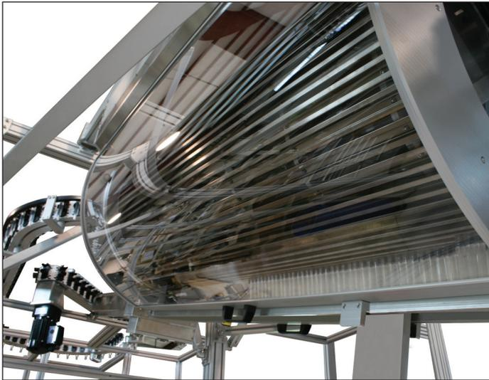
**Figure 4: Syringe accumulator.**
