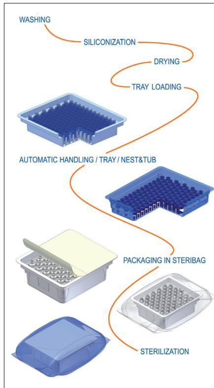
**Figure 2: Schematic workflow of the *EZ-fill™* process.**
