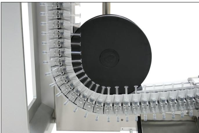
Figure 2: Non-contact conveying.
