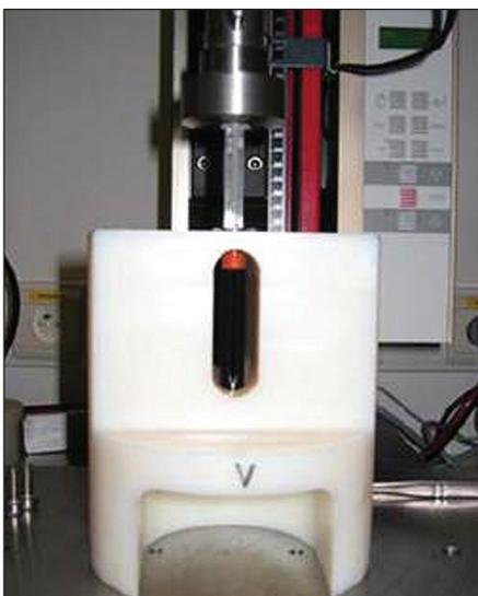
**Figure 3: PBSE, Build-Up for Compression Testing.**
