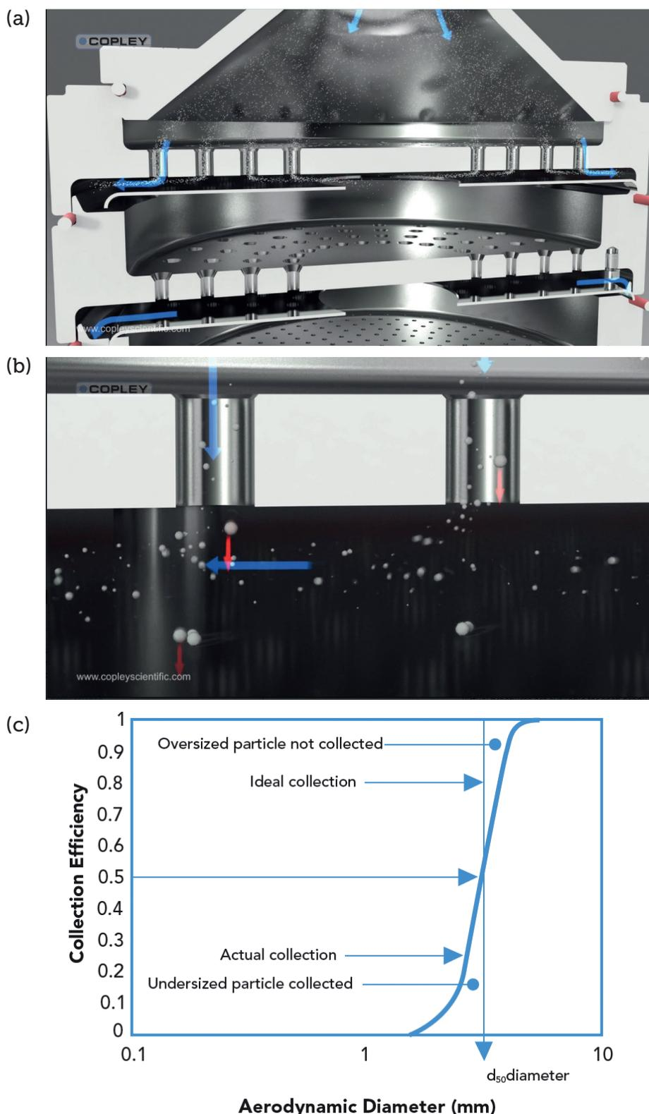
Figure 1: As sample is drawn through the stages of a cascade impactor (a), progressively smaller particles acquire sufficient inertia to break free of the prevailing air flow and impact on the associated collection surface (b). At any given flow rate each stage therefore has a defined cut-off diameter, the D50 of the collection efficiency curve (c).
