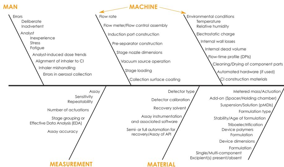
Figure 3: The complexity and manual nature of cascade impaction means that there are many potential sources of variability.<sup>5</sup>
