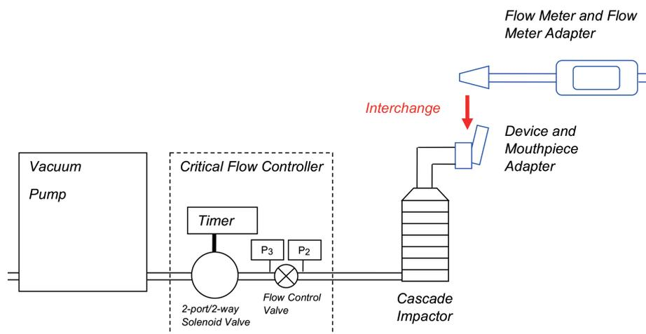
Figure 4: For all OIPs, test flow rate can be determined by replacing the OIP with a flow meter and adjusting the flow control valve. Critical flow across this valve (P3/P2 ratio  $\leq 0.5$ ) is an additional requirement for DPIs, which are most easily set-up using a critical flow controller.
