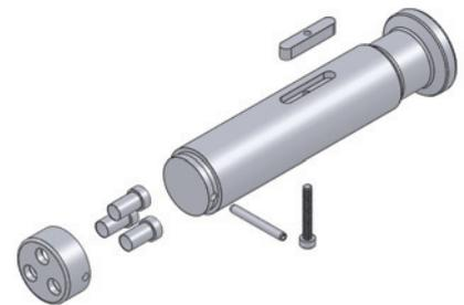
Figure 1: Assembly configuration comprising the punch body, cap, and individual punch tips.
