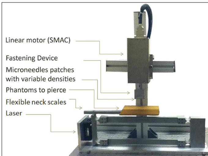
Figure 2: The test bench.
