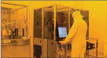
**Figure 6: Nanoject™ manufacture and assembly takes place in ISO class 5 down to ISO class 3 clean rooms.**
