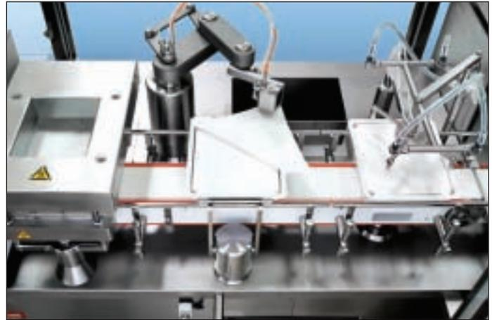
**Figure 2: Fully automatic tub opening (ATO). Smooth and low particle opening process.**
