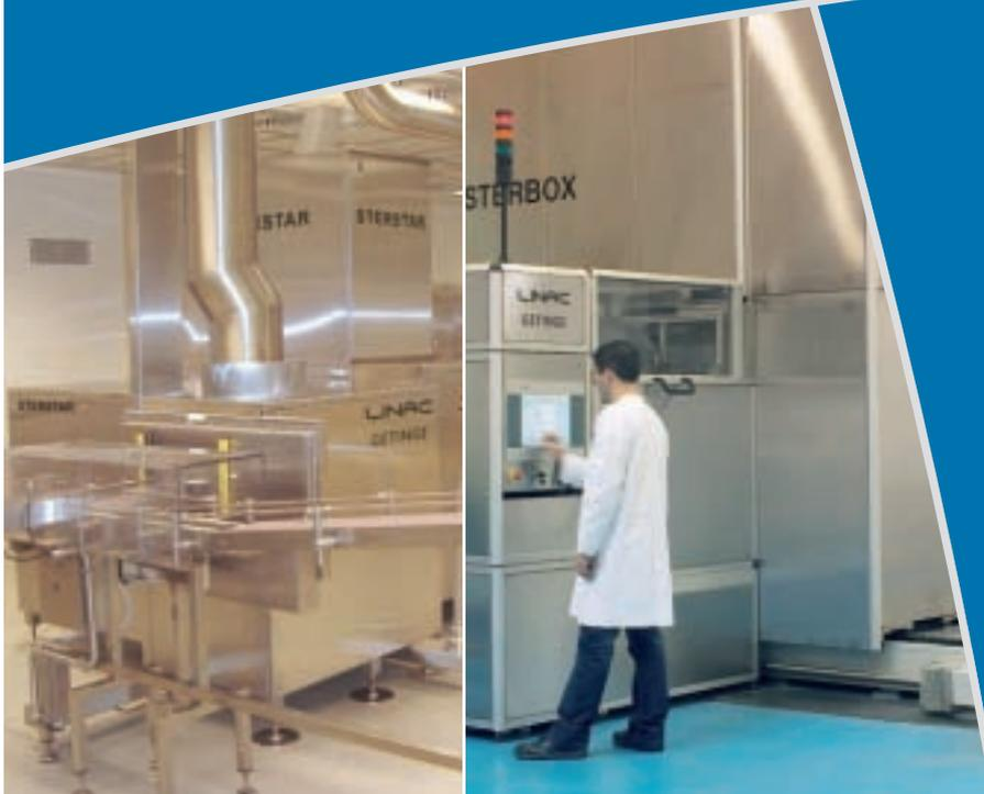
In-line stand-alone sterilisation tunnels using electron beam for surface sterilisation (**SterStar™**) and core sterilisation (**SterBox™**).
