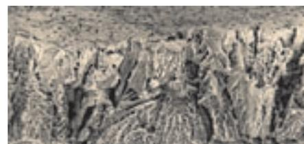
**Figure 1: Magnified cross section of a lyophilised ODT, showing the highly porous structure**
