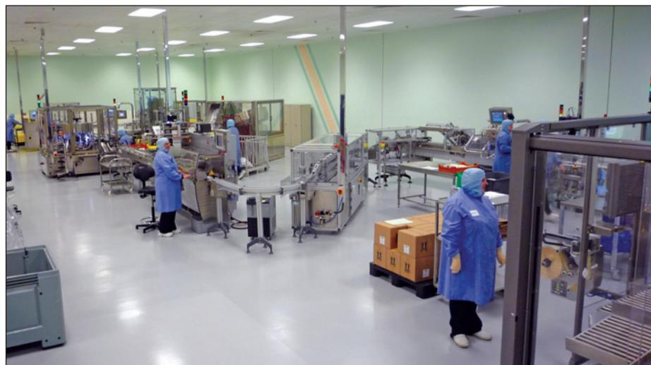
**Figure 4: High speed automated packing line.**
