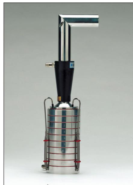
**Figure 3: Use of a mixing inlet decouples flow through the test device from flow through the impactor extending options for more relevant inhaled product testing.**
