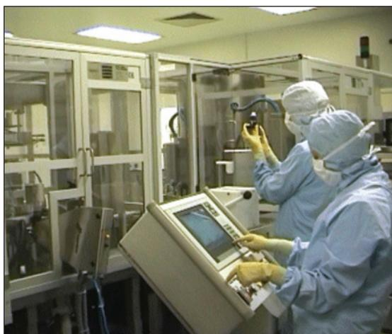
**Figure 2: DPI filling and final assembly equipment.**
