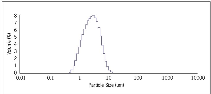
**Figure 3: Particle size distribution of Technosphere®/Insulin particles measured by laser diffraction. 90% of the particles are below 5.7 μm in diameter; 50% of the particles are below 2.6 μm in diameter, 10% of the particles are below 1.1 μm in diameter.**
