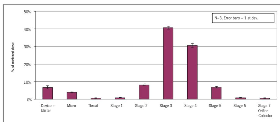
Figure 3: NGI performance of a DPI formulation containing 400 $\mu\text{g}$  apomorphine hydrochloride in a 2mg formulation, delivered from the Aspirair active DPI device.
