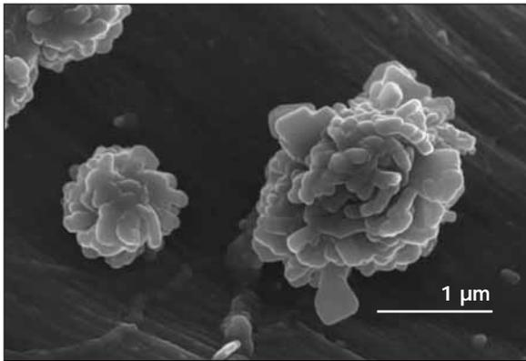
**Figure 2: Scanning electron micrograph of Technosphere® particle**
