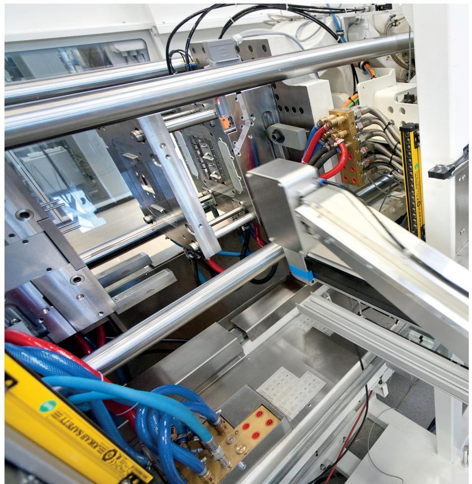
**Figure 3:** If the Z.NFS is integrated into the Z.BLIZZARD as shown here, it is an integrated system that guarantees the highest level of purity in the production process, as there is no human touch and the process can be carried under cleanroom conditions.
