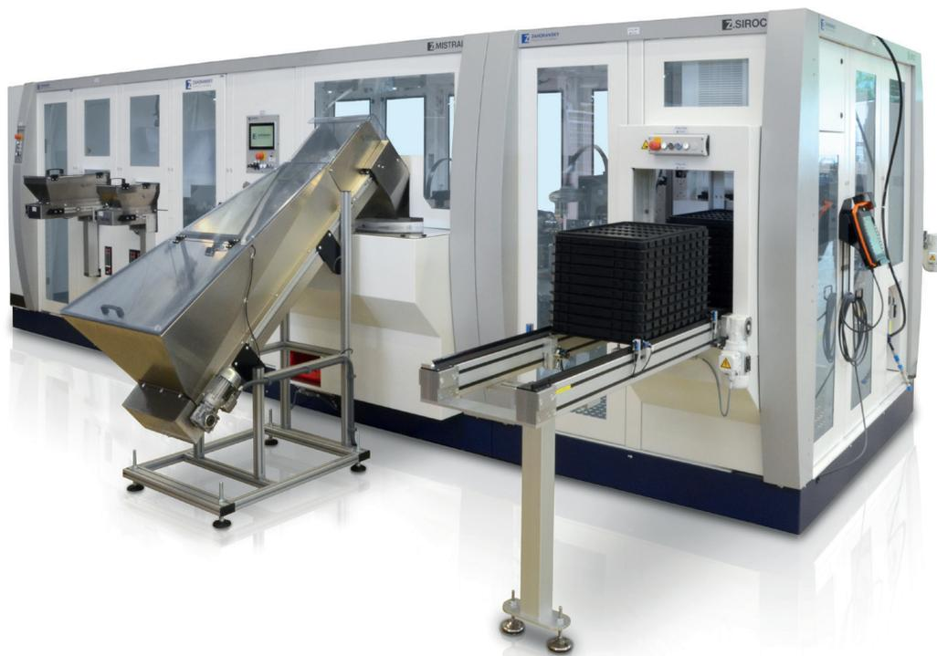
Figure 4: If the Z.BLISSARD is still connected to the Z.MISTRAL, which is responsible for the downstream, and the palletising system Z.LODOS, it is possible to cover the complete process chain, from the granulate to the finished packed PFS.
